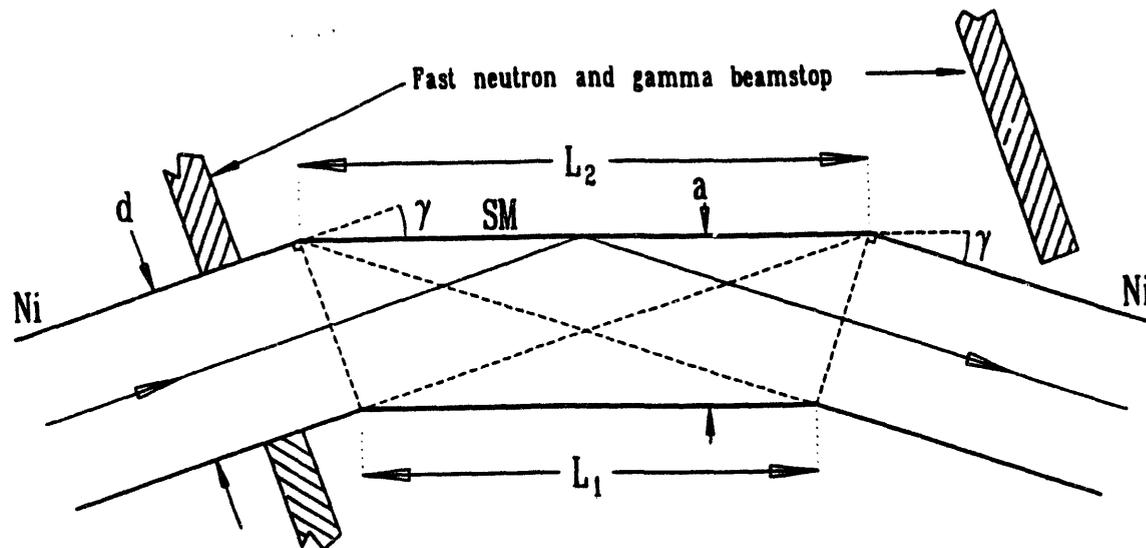
Fig 1. Plan view of an optical filter geometry
