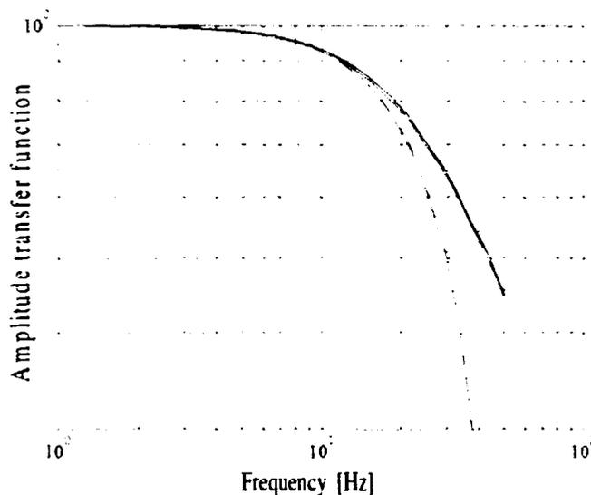
**Figure 4** The amplitude transfer functions of an analogue 1st order low pass filter (solid curve) and of a digital filter obtained from the improved difference equation (11) (dashed curve).
