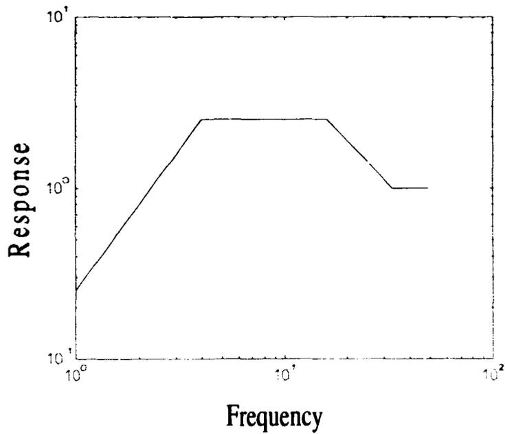
**Figure 7** The Standard Response Spectrum according to IEEE 344
