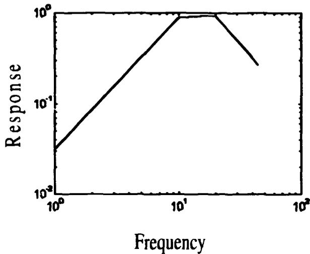
**Figure 15** A response spectrum suggested for a typical hard rock site in Sweden.
