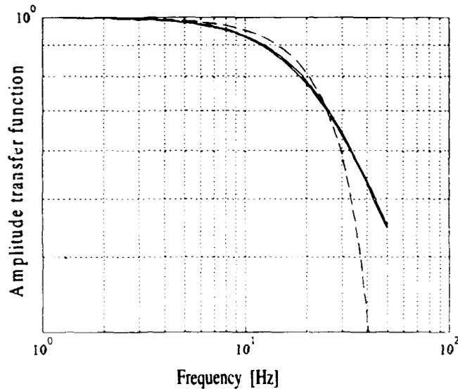
**Figure 5** The amplitude transfer functions of an analogue 1st order low pass filter (solid curve) and of a digital filter obtained from the improved difference equation (11) and prewarping (dashed curve).
