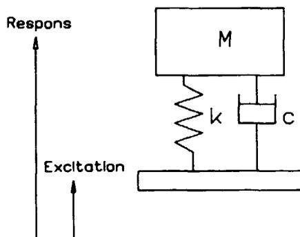
**Figure 1:** A schematic sketch of a Single Degree of Freedom System
