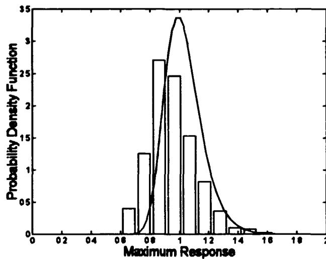
Figure 13 The maximum responses obtained at 1000 simulations (the histogram) together with the predicted probability density function of maximum responses.
