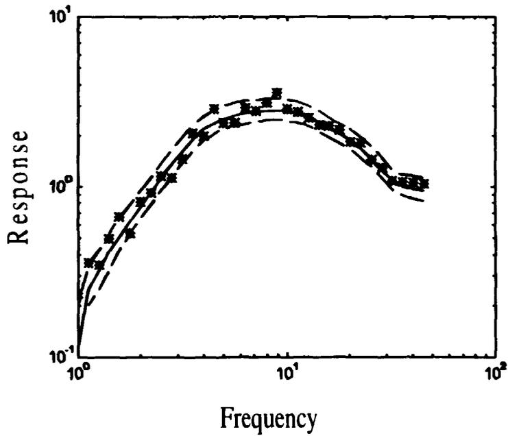
**Figure 11** A response spectrum obtained after one simulation (asterisks) together with the predicted spectrum (solid line) and the 5% and 95 % prediction limits (dashed lines).
