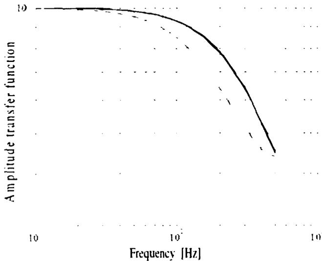
**Figure 3** The amplitude transfer functions of an analogue 1st order low pass filter (solid curve) and of a digital filter obtained from the simple difference equation (7) (dashed curve).
