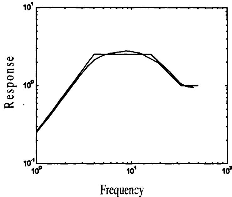
**Figure 9** The predicted response spectrum after filtering white noise with the filter shown in Figure 8. The prediction was performed by the simple approach. The straight lines show the target spectrum (SRS according to IEEE 344).
