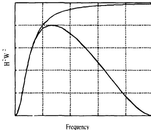
**Figure 6** The square of the amplitude transfer function times the square of the frequency as a function of the frequency for an analogue 1st order low pass filter (upper curve) and its corresponding frequency warped digital filter (lower curve)
