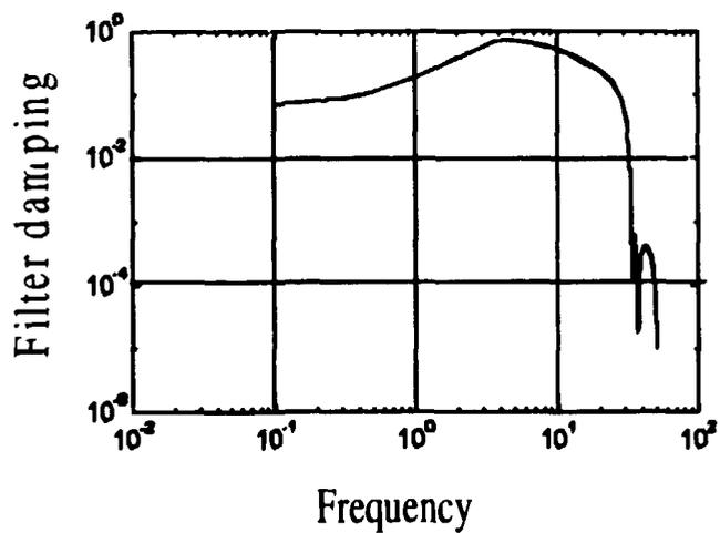
**Figure 8** The digital band pass filter used for generating time histories with response spectrum according to IEEE 344
