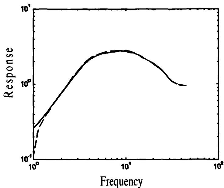
**Figure 10** A comparison between predicting the response spectrum by the simple approach (dashed line) and by using the Poisson approximation (solid line).
