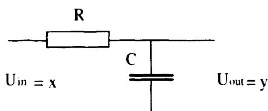
Figure 2: An electrical network that can be used as a low-pass filter
