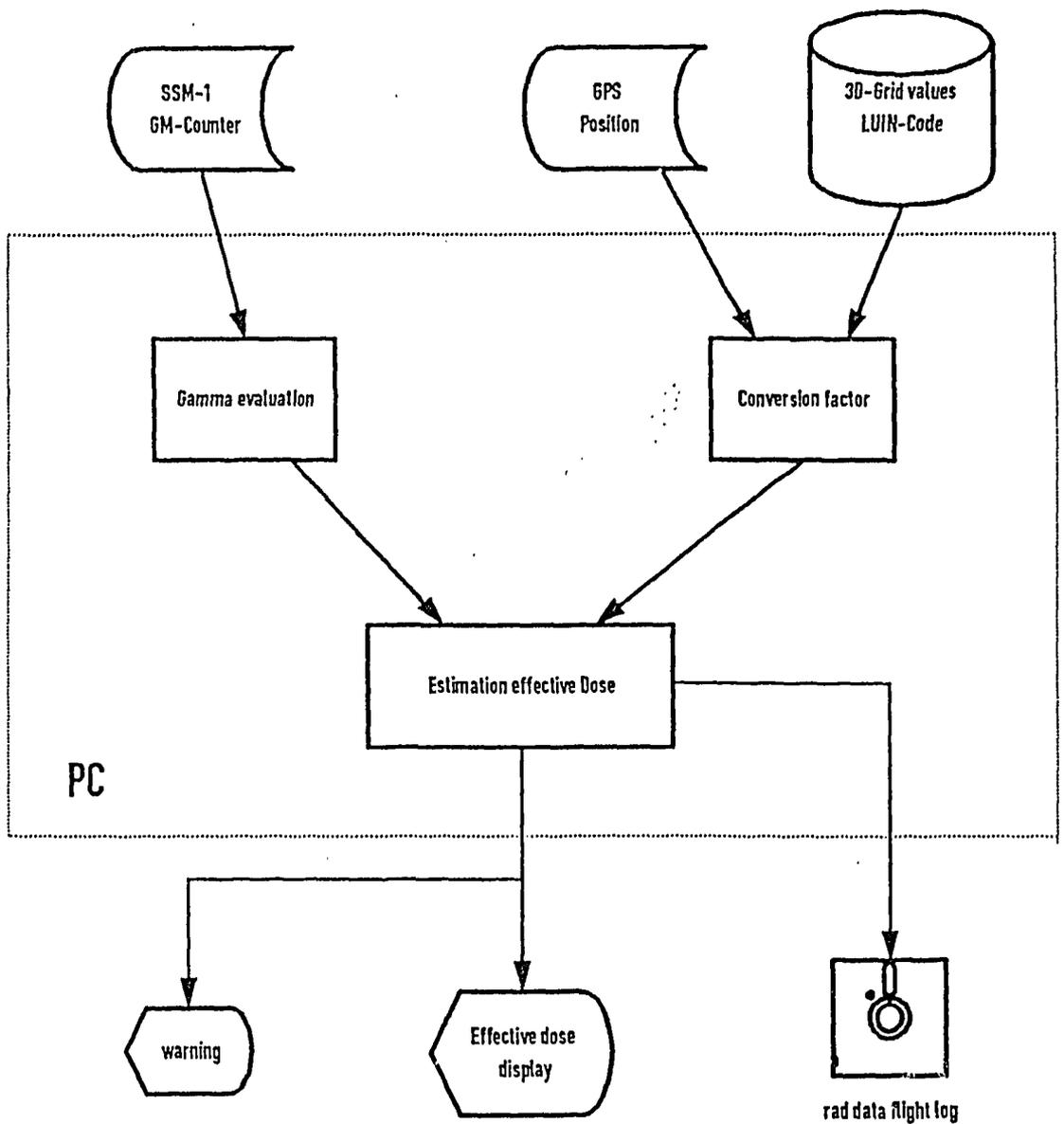
Figure 4. Design Concept of the ACREM Aircrew Radiation Exposure Measuring System
