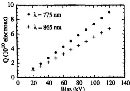
**Figure 4:** Charge limit versus cathode bias for two laser wavelengths.
