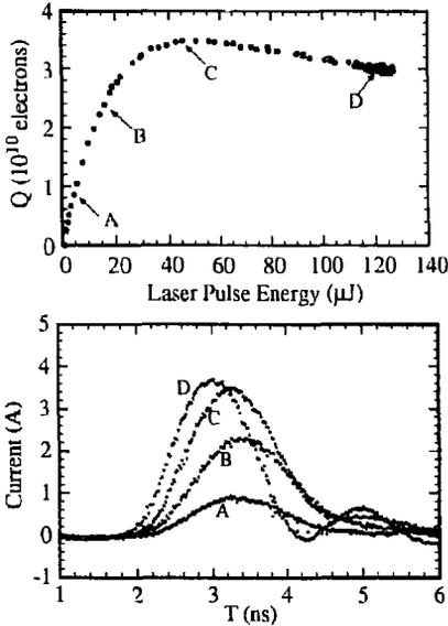
**Figure 1:** Photoemitted charge versus laser pulse energy (upper panel) and representative charge pulse shapes (lower panel) at several laser pulse energies.
