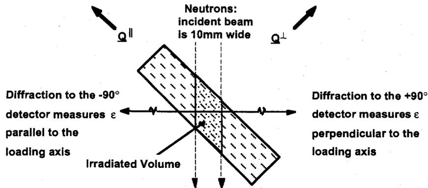
Figure 1 Schematic of specimen orientation in the NPD for a uniaxial load experiment (the backscattering detectors are not shown).
