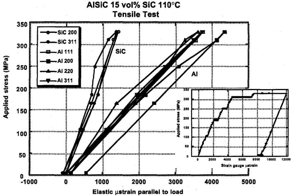
Figure 2: Parallel strain relative to initial material state in a uniaxial tension test of a 15 vol% SiC Al 6091 (T6) particulate MMC.
