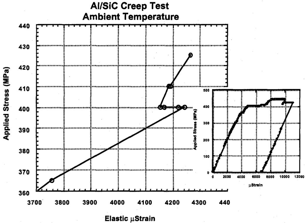
Figure 3: Parallel elastic composite macrostrain relative to initial material state in a uniaxial tension fracture test of a 15 vol% SiC Al particulate MMC. Data were taken in 60 minute intervals at a given load.
