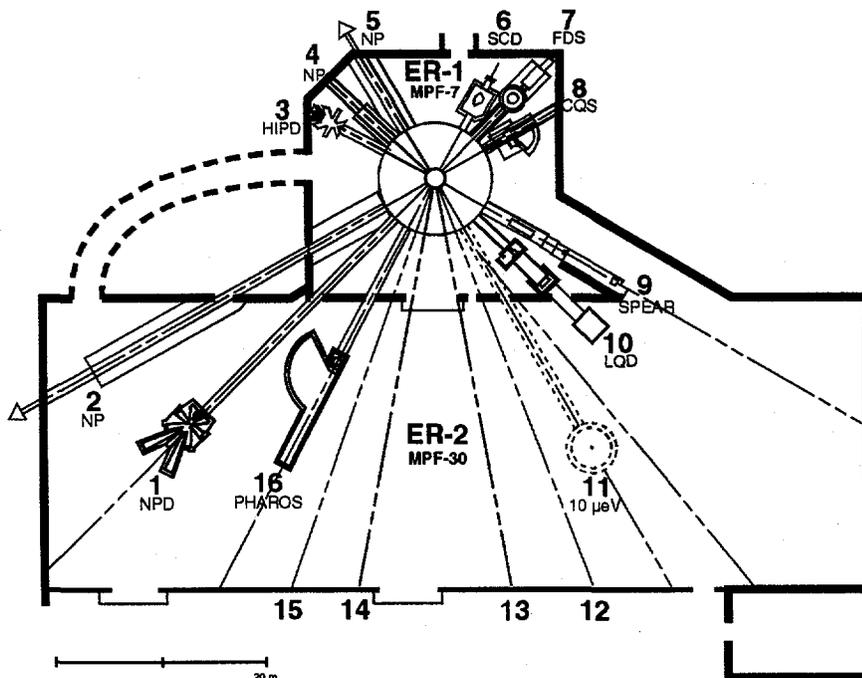
**Figure 3.** Layout of the instrument suite in the two adjacent LANSCE experiment rooms. NPD, HIPD, SCD, LQD, FDS, SPEAR, and PHAROS (Phase I) are established instruments and are part of the LANSCE user program. PHAROS (Phase II), the Protein Crystallography Diffractometer, and the 10- $\mu\text{eV}$  Spectrometer are under construction. The flight paths for the beams are numbered from 1 to 16.
