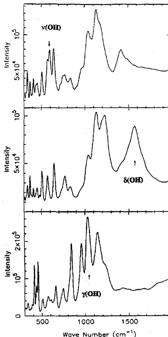
**Figure 6.** Oriented single crystal vibrational spectra obtained on FDS. The orientations of  $Q$  are (top to bottom): parallel to H-bond; perpendicular in-plane; and perpendicular out-of-plane (of the molecule).
