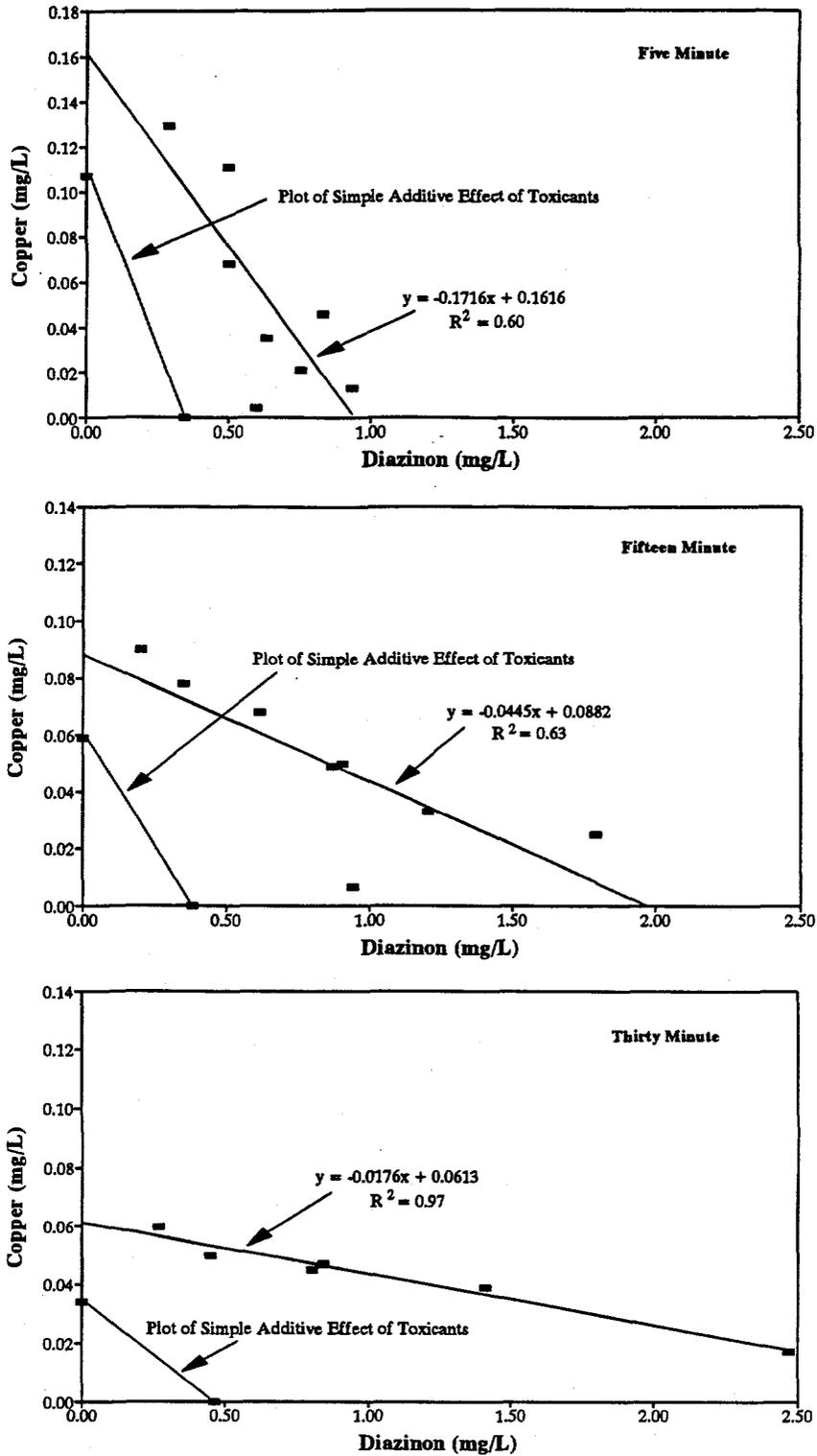
Figure 5. Five, Fifteen, and Thirty Minute EC50's for Copper and Diazinon Using the Microtox™ Sucrose-Based Assay.
