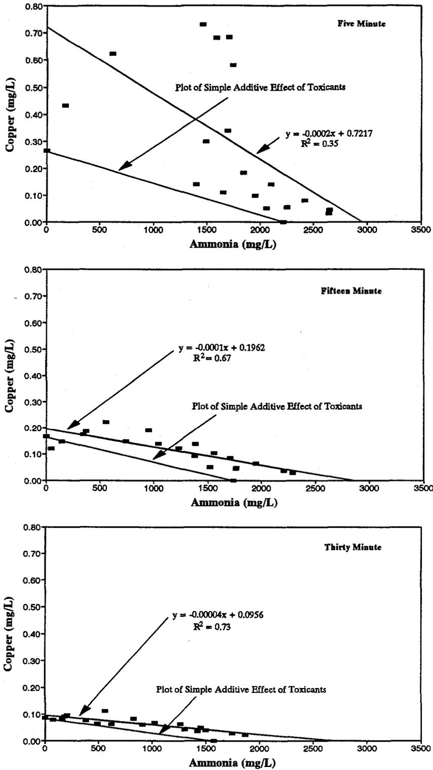
Figure 1. Five, Fifteen, and Thirty Minute EC50's for Ammonia and Copper Using the Microtox™ Basic Test Protocol.
