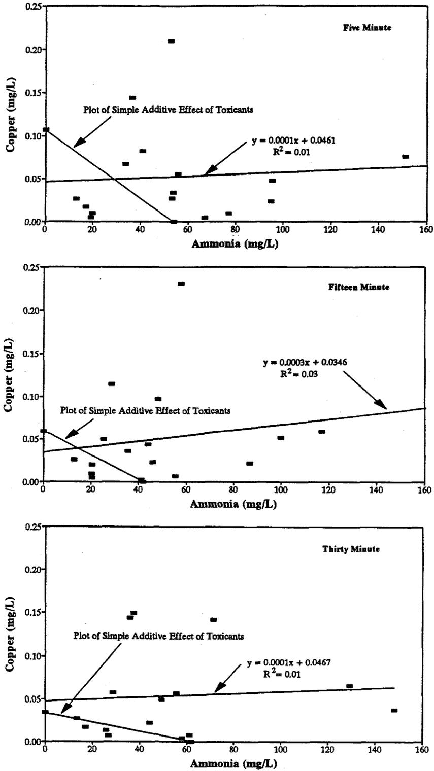
Figure 4. Five, Fifteen, and Thirty Minute EC50's for Ammonia and Copper Using the Microtox™ Sucrose-Based Assay.
