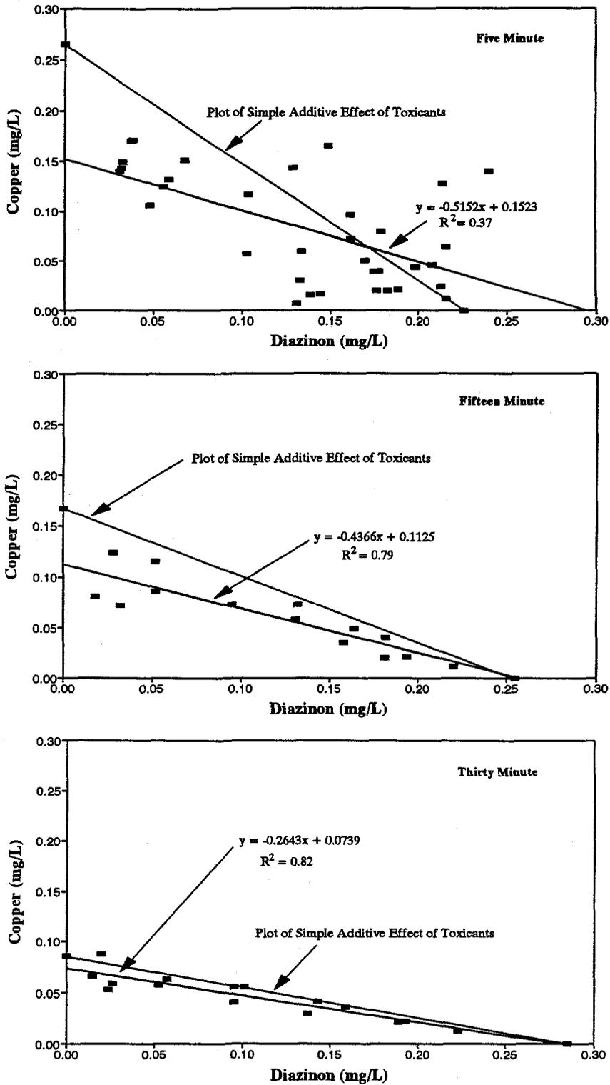
Figure 2. Five, Fifteen, and Thirty Minute EC50's for Diazinon and Copper Using the Microtox™ Basic Test Protocol.
