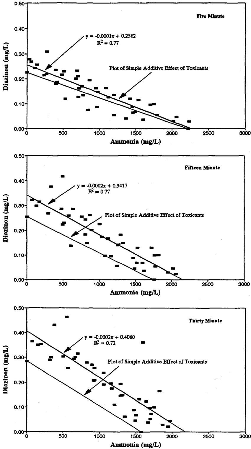
Figure 3. Five, Fifteen, and Thirty Minute EC50's for Ammonia and Diazinon Using the Microtox™ Basic Test Protocol.
