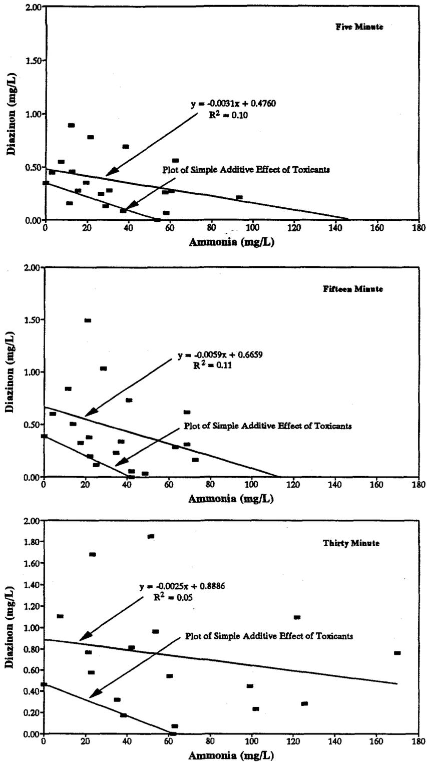
Figure 6. Five, Fifteen, and Thirty Minute EC50's for Ammonia and Diazinon Using the Microtox™ Sucrose-Based Assay.
