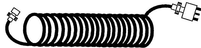
SJEO HEAVY DUTY RETRACTILE ELECTRICAL CORD, #12, 3 WIRE, PART# 7520K23, ONE END AMPHENOL STRAIGHT PLUG MALE 5 PIN MS3106A 14S-5P "636", AN3057 "636" CABLE CONNECTOR WITH TELESOPING BOOT, OTHER END 120VAC STANDARD 3 PIN RECEPTACLE PLUG, (AMPHENOL END) LAND BLACK WIRE ON PIN #1, WHITE WIRE ON PIN #2 AND GREEN WIRE ON PIN #3, OTHER END LAND BLACK WIRE ON HOT SCREW, WHITE WIRE ON NEUTRAL SCREW AND GREEN WIRE ON GROUND SCREW
