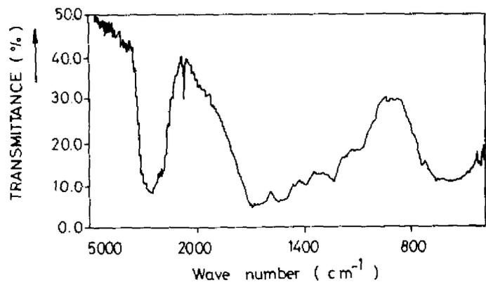
FIG.4. TRANSMITTANCE SPECTRUM OF LYSOZYME SAMPLE OBTAINED AFTER DIVIDING SPECTRUM IN FIG.3. BY SPECTRUM IN FIG.2.
