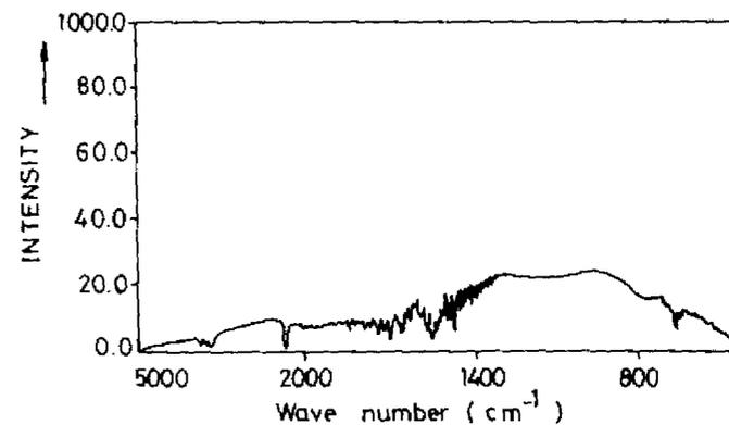
FIG.2. FOURIER TRANSFORM OF THE INTERFEROGRAM SHOWN IN FIG.1; THE SINGLE CHANNEL REFERENCE POWER SPECTRUM MEASURED THROUGH THE EMPTY COMPARTMENT.
