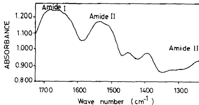
FIG.5. ABSORPTION SPECTRUM OF LYSOZYME SAMPLE FROM 1700  $\text{cm}^{-1}$  TO 1300  $\text{cm}^{-1}$  SHOWING AMIDE I, AMIDE II AND AMIDE III SPECTRAL REGIONS.
