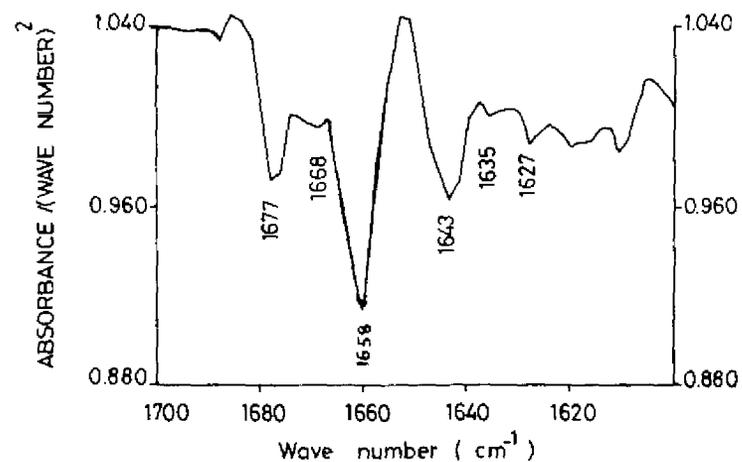
FIG.6. SECOND - DERIVATIVE FTIR SPECTRUM OF LYSOZYME IN THE AMIDE I REGION FROM 1700  $\text{cm}^{-1}$  TO 1600  $\text{cm}^{-1}$ .
