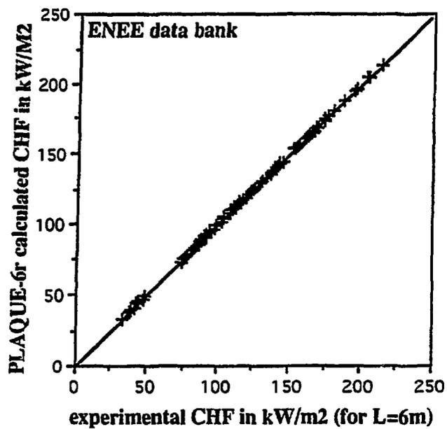
Figure 3- Comparison between calculations with PLAQUE-6r and measured CHF
