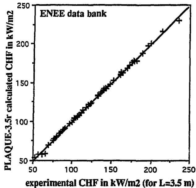
Figure 4- Comparison between calculations with PLAQUE-3.5r and measured CHF
