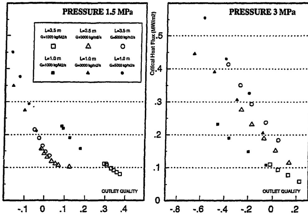
Figure 1 - Measured CHF on DEBORA for two different heating lengths
