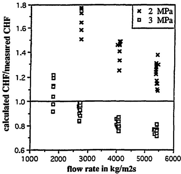
Figure 11- Calculations with Weisman & Pei model to experimental data ratio versus mass velocity
