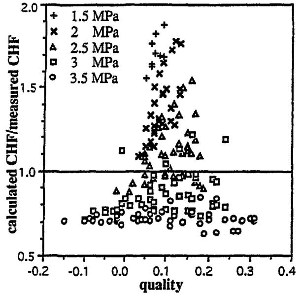
Figure 10- Calculations with Weisman & Pei model to experimental data ratio versus quality
