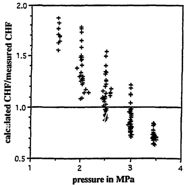
Figure 12- Calculations with Weisman & Pei model to experimental data ratio versus pressure
