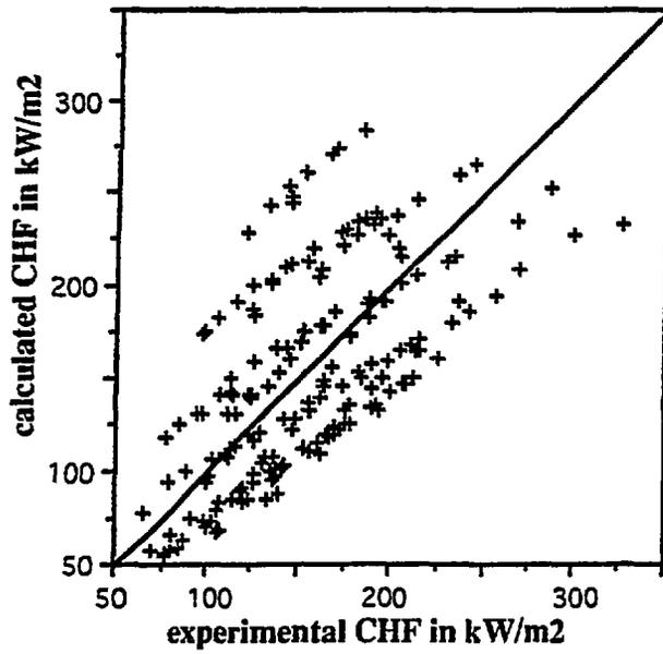
Figure 9- Comparison between calculations with Weisman & Pei model and experimental data
