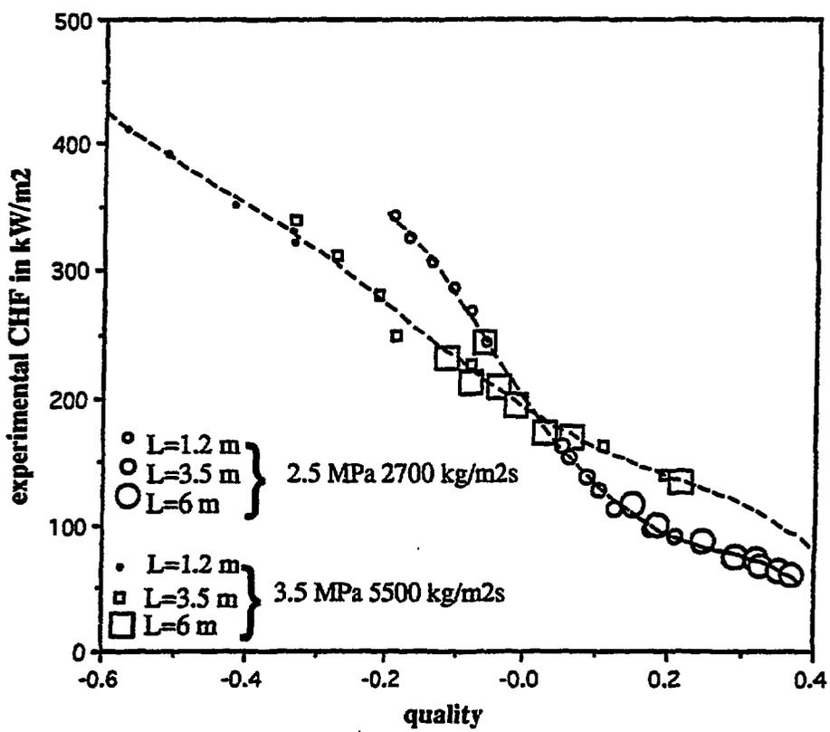
Figure 2 - Experimental CHF versus quality for ENEE experiments.
