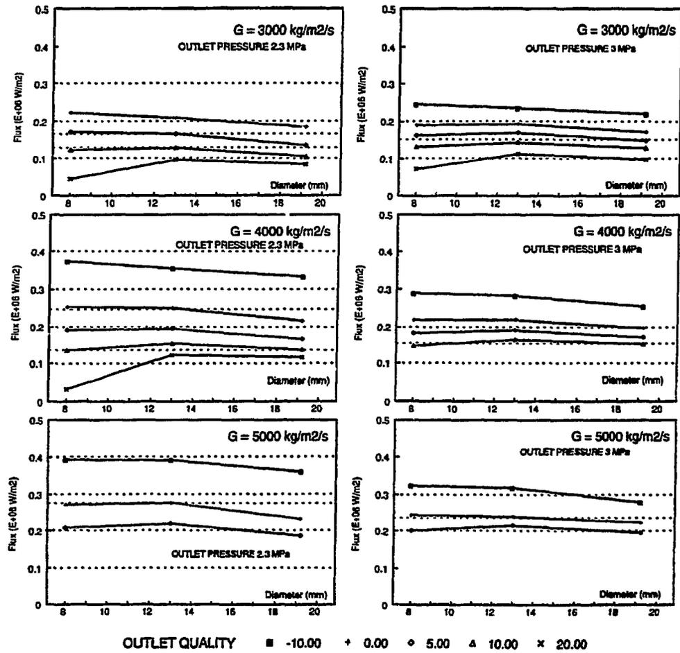
Figure 8 - Measured CHF versus tube diameter as interpolated by PLAQUE
