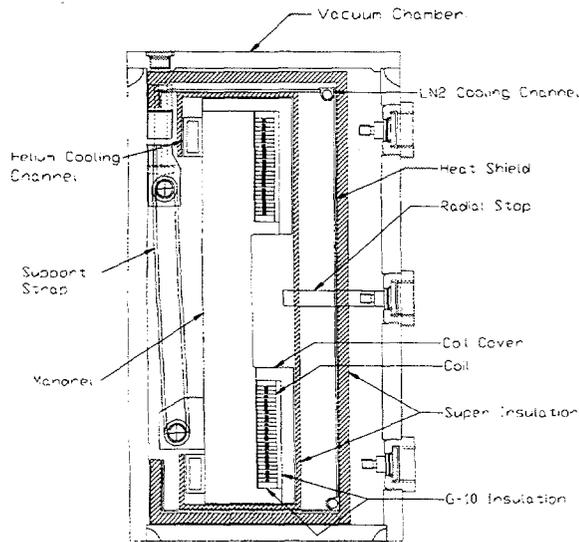
Fig. 4 Cross-section of Outer Cryostat Assembly
