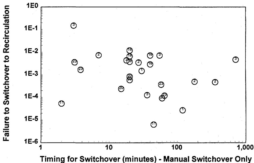
Figure 7. HEPs for Switchover to Recirculation as a Function of Time Available for the Switchover
