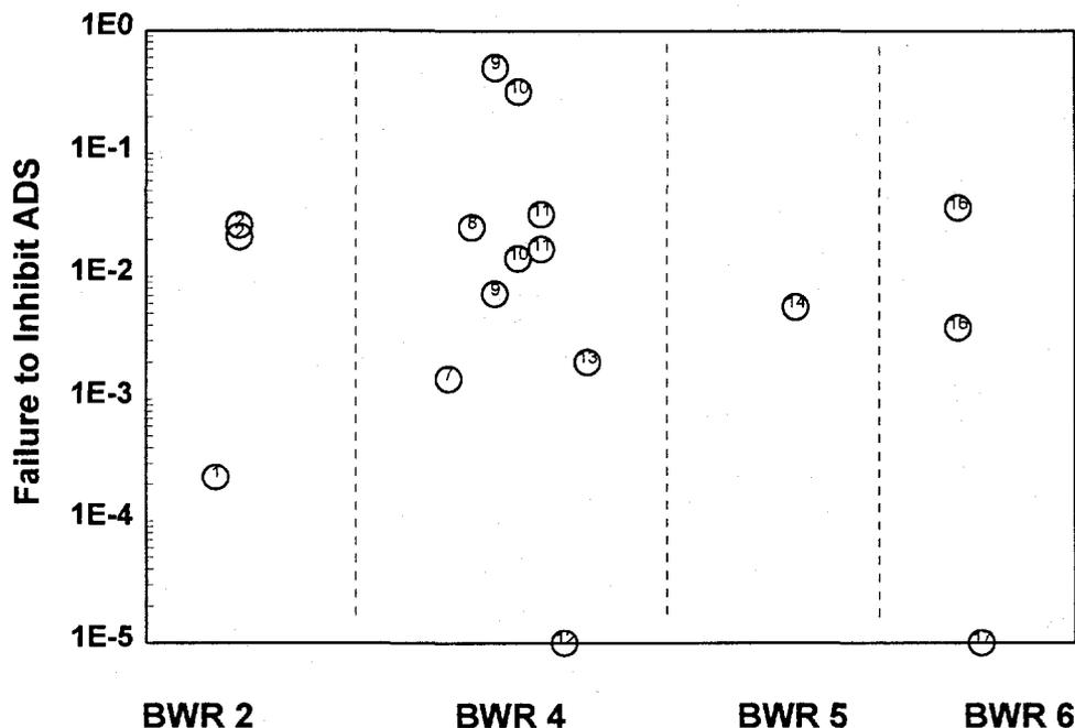
Figure 10. HEPs for Inhibition of ADS by BWR Type
