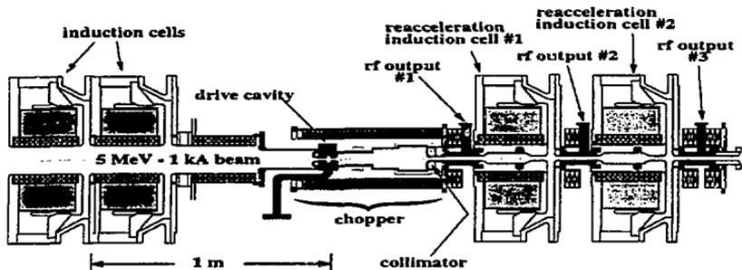
FIGURE 2. Layout of reacceleration experiments at LLNL.
