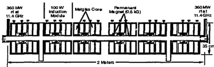
FIGURE 5. 2-m module in the main TBA.
