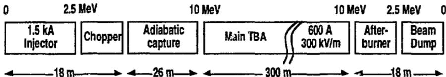
FIGURE 4. Schematic of one RK-TBA unit.
