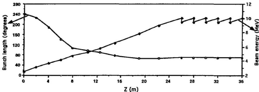
FIGURE 12. Evolutions of bunch length and kinetic energy of a beam bunch during the "adiabatic capture" process illustrated in Fig. 11.
