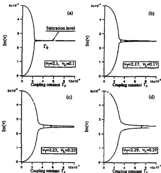
**Figure 5.** Imaginary part of the eigenvalues describing longitudinal and transverse motion as a function of the coupling strength between the modes. The bunching and coupling cavities are next to each other and  $180^\circ$  from the laser cooling section. The longitudinal and transverse tunes are varied in the four figures, keeping the resonance condition satisfied. The damping rate was held fixed such that  $\Lambda_d/2\pi=0.01$ .
