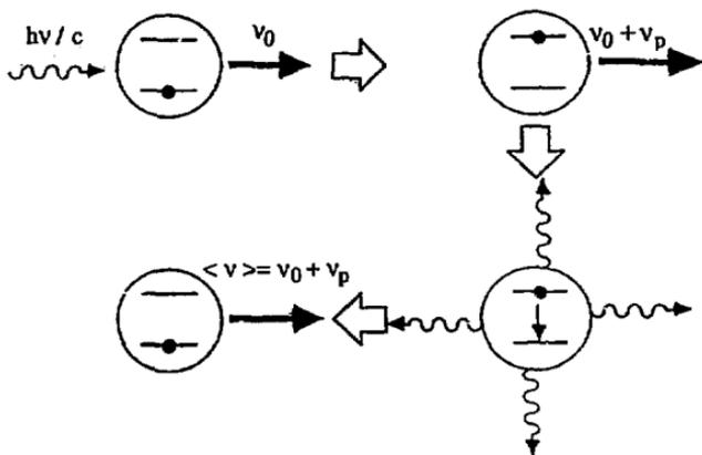
FIGURE 1. The principle of laser cooling.
