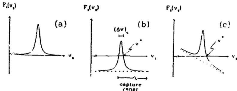
FIGURE 3. (a) The spontaneous force itself has no stable point  $v^*$ . With the help of (b) constant or (c) linear auxiliary force  $F_{aux}$  (dashed lines), such a point can be generated for the combined forces (solid line).
