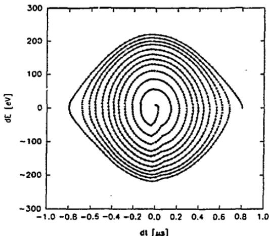
FIGURE 4. Longitudinal phase space plot illustrating the principle of bunched-beam laser cooling. Energy deviation and time deviation are plotted for a single particle in an RF bucket.
