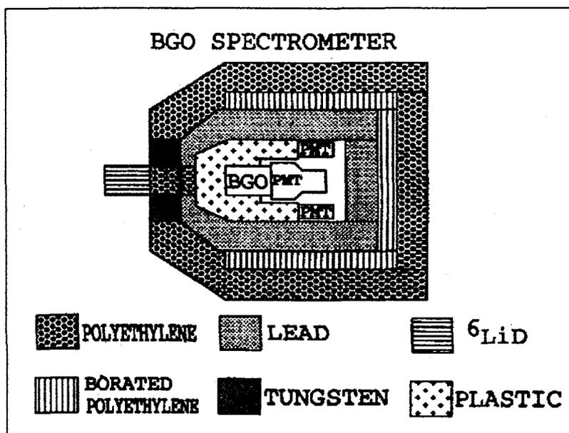
Figure 1. Diagram of the 10 by 15 cm BGO detector with active and passive shielding.
