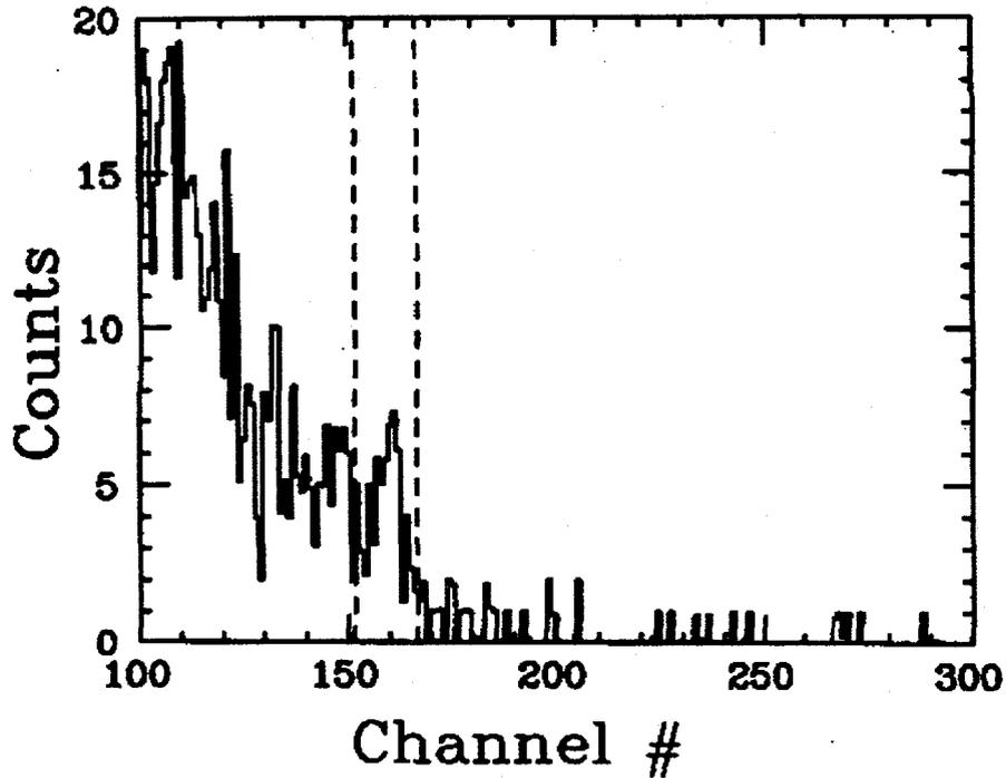
Figure 5. Spectrum at  $125^\circ$  from the  $^{40}\text{Ca}(n,\gamma)$  experiment. The dashed lines indicate the region of the peak due to  $\gamma$  rays from capture to the ground state. The data are for an incident neutron energy of 10.3 MeV and a neutron energy bin width of 50 keV. The data below the ground state capture peak include both neutron and  $\gamma$ -ray events.
