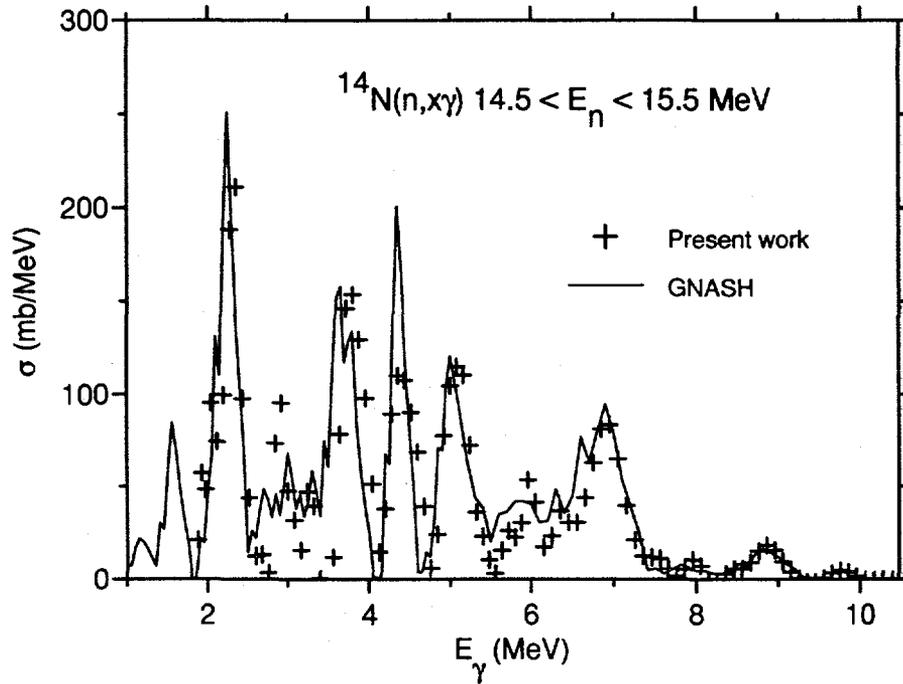
Figure 3. The  $\gamma$ -ray spectrum for  $N(n, x\gamma)$  at  $E_n = 15$  MeV. The solid line is a GNASH model calculation.<sup>11</sup>
