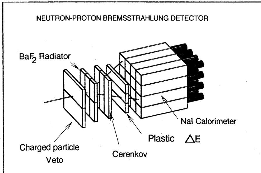
**Figure 2.** Schematic diagram of the  $\gamma$ -ray telescope. The individual NaI elements measure 10 by 10 by 40 cm. Timing, position, and particle-type information are used to select positron-electron pairs produced in the radiator.
