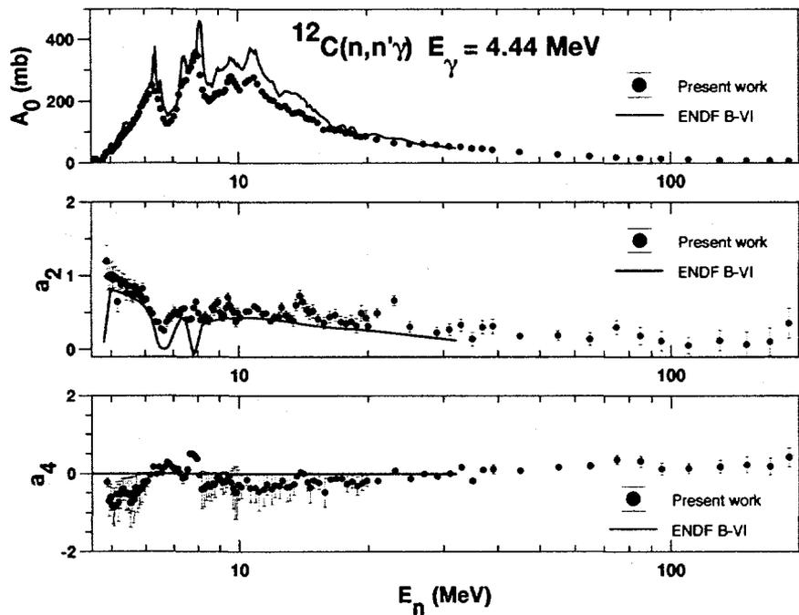
Figure 4. The excitation function for the 4.44 MeV  $\gamma$  ray from  $C(n, n'\gamma)$ . The solid line is the ENDF B-VI evaluation.
