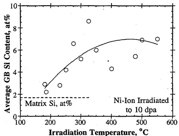
Figure 9. Irradiation Temperature Effects on the Grain Boundary Silicon Content.
