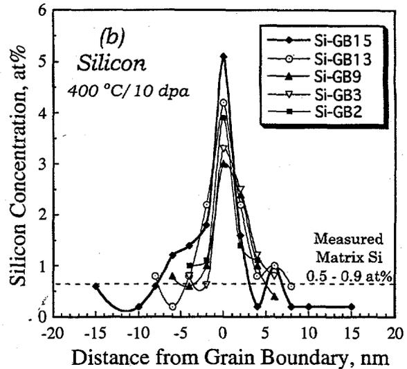
Figure 3. STEM-EDS Measured Composition Profiles for Cr (a) and Si (b) Across Various High-Angle Grain Boundaries in the Ion-Irradiated FeNiCr Alloy.
