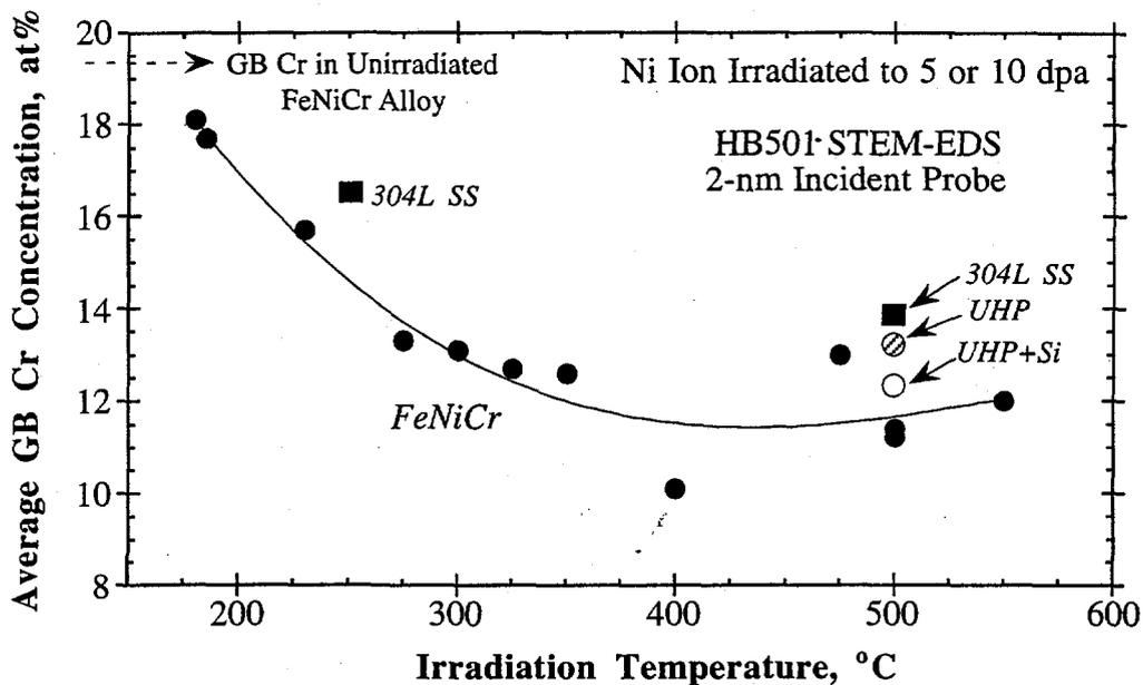
Figure 7. Irradiation Temperature Effects on the Grain Boundary Cr Concentration. Most Irradiations at a Dose of 10 dpa Except for Several Points at 500°C.
