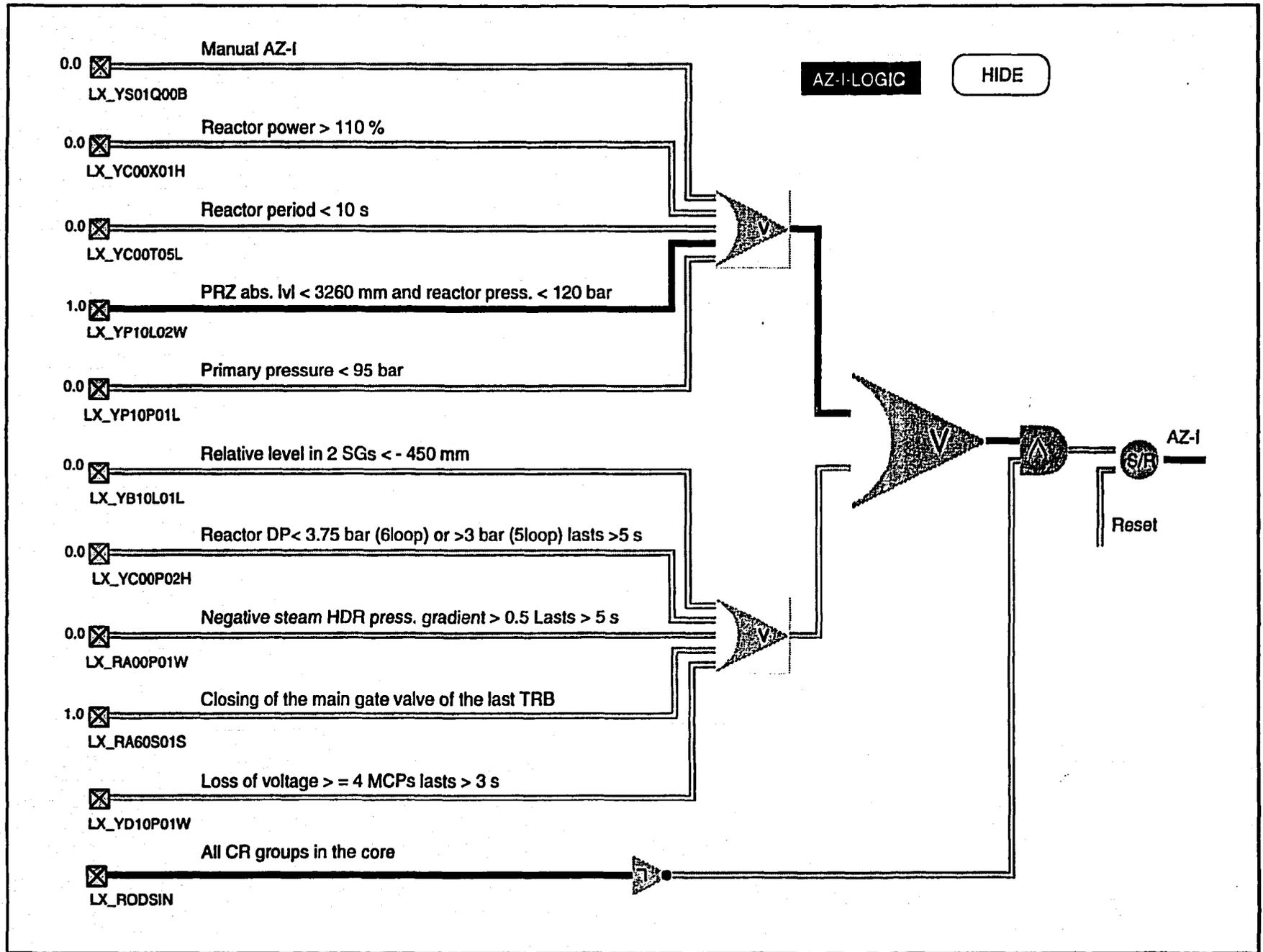
Figure 4. RP level I logic diagram
