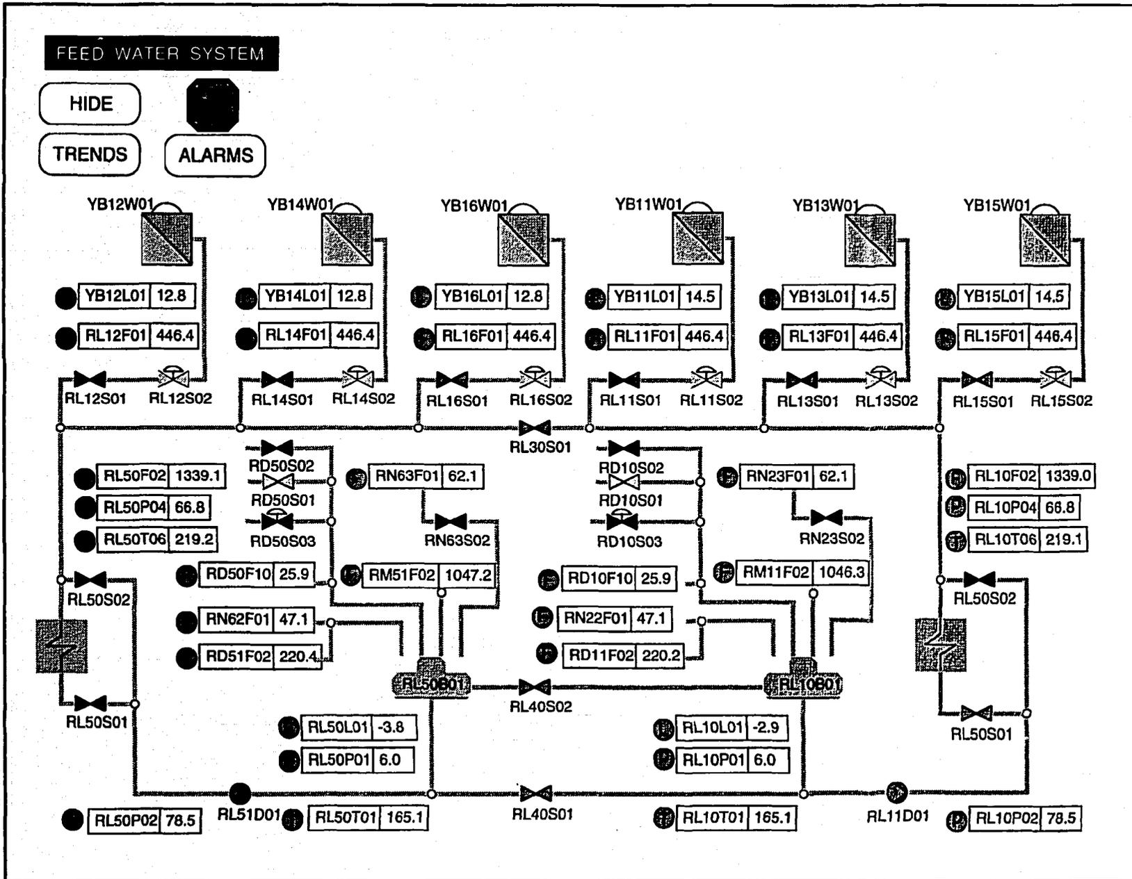
Figure 3. Feedwater system picture in GPCS
