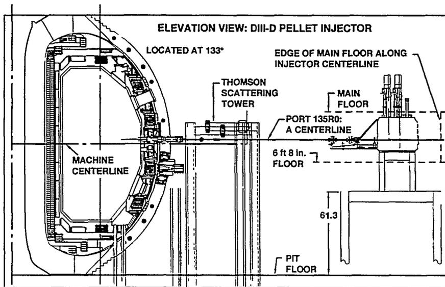
Figure 1. Schematic of three-barrel injector installation on DIII-D.
