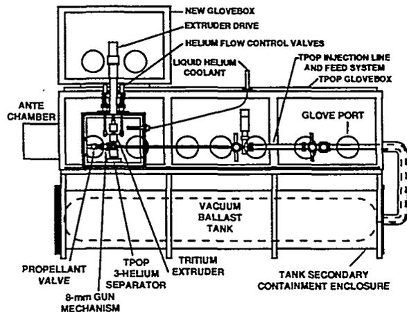
Figure 3. Schematic of TPOP II experiment.
