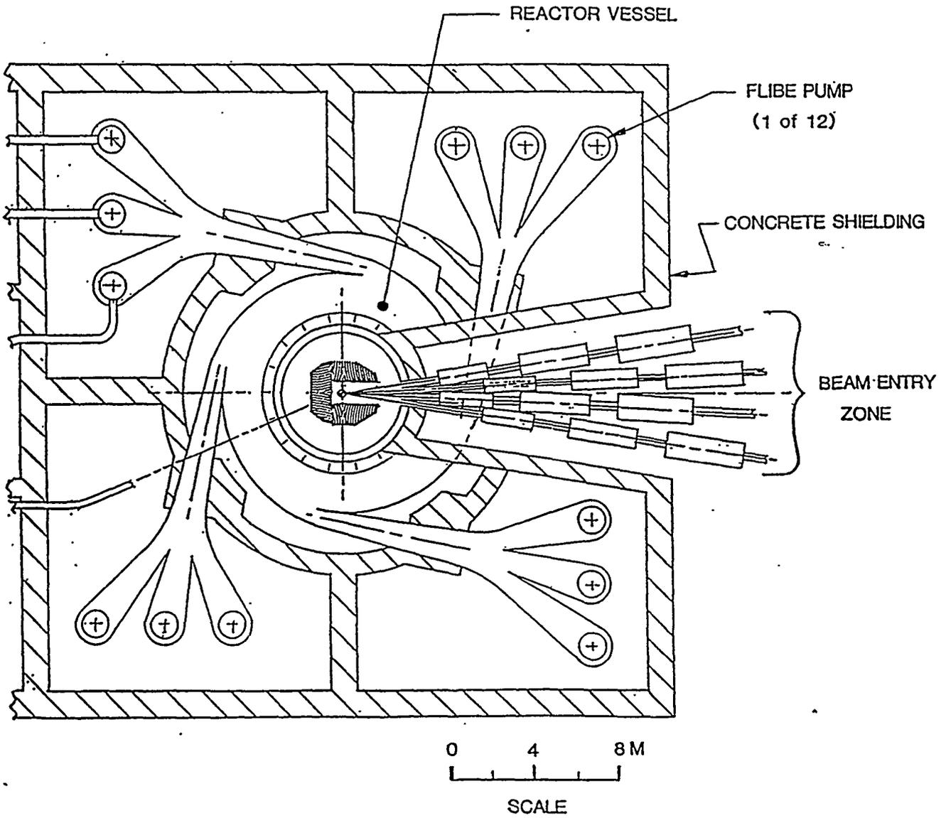
FIGURE 7. REACTOR BUILDING - PLAN VIEW
