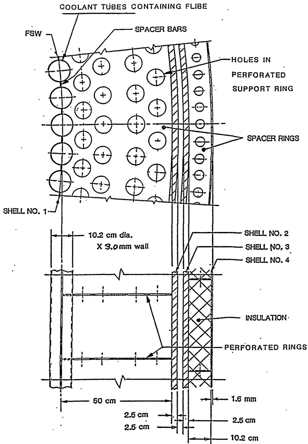
FIGURE 3 VESSEL WALL CONSTRUCTION
