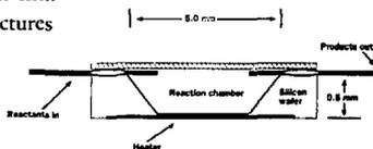
**Prototype chemical-reaction chamber etched into a silicon wafer.** The chamber is just one component of a miniature microflow system, essentially a “chemical plant on a chip.” Other components include tiny ultrasonic pumps, mixers, and resistive heaters—each the size of a few grains of sand.
