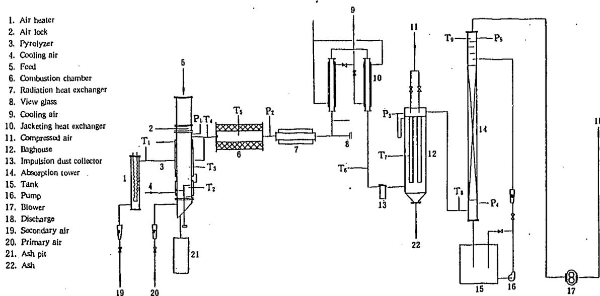
Fig. 1 The flow sheet of pyrolysis incineration
