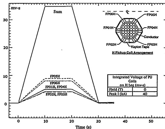
Fig. 5. Measurement of current distribution around H Leg at zero field
