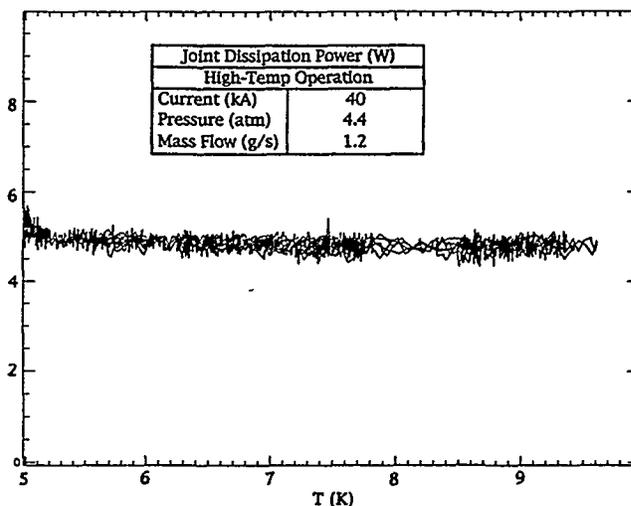
Fig. 7. Power dissipation of the lower joint up to 9K
