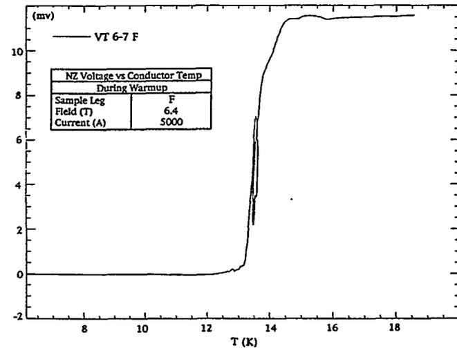
Fig. 2. Measurements of NZ Voltage of F Leg
