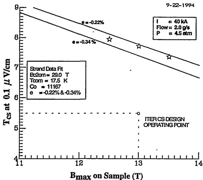
Fig. 3. Measured Tcs for F Leg
