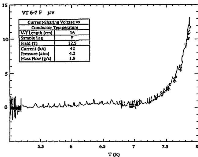
Fig. 4. Measured Current-Sharing Curve for F Leg
