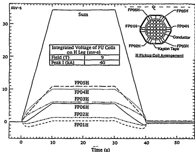
Fig. 6. Measurement of current distribution around H Leg at 9 T
