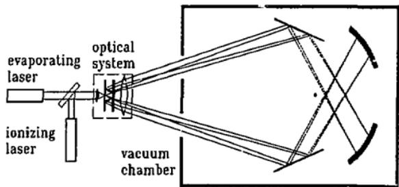
*Fig. 4.* Schematic of the CATRION laser source.
