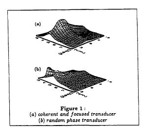
Noise reduction potential in single scattering: in a classical (coherent) processing, the signal-to-noise ratio (SNR) is rather low: 1.91 or 1.0 respectively for the envelope- and the intensity-detected signals [11]. We derive a general expression for the SNR obtainable in totally incoherent pulse echo processing. After a set of RPS positions, the SNR magnitude is defined as [6]:  $SNR_{magnitude} =$
