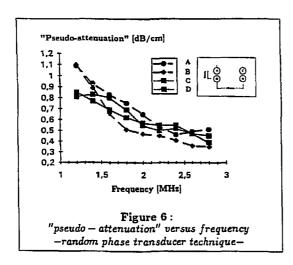
Discussion about "attenuation" and "pseudo-attenuation": the results issued from the spatial compounding technique are homogeneous as expected because the scanned areas are larger than the mean grain size (5mm).
