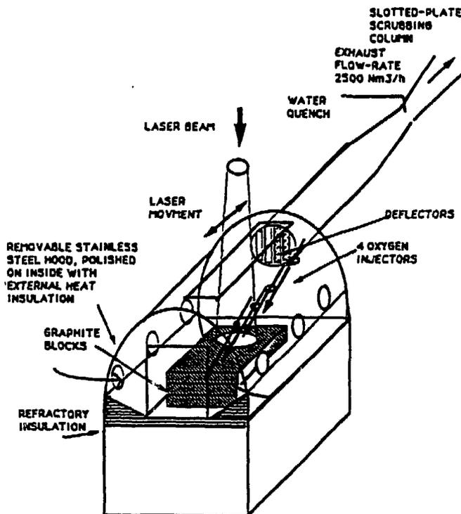
Figure 6. Pilot laser furnace schematic
