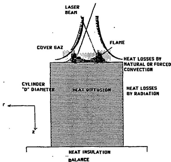
Figure 2. Experimental configuration
