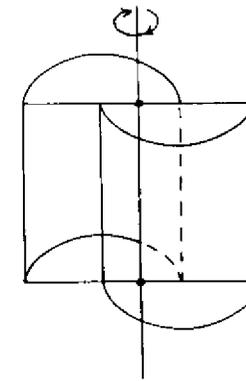
Fig. 1 The Savonius windmill.
