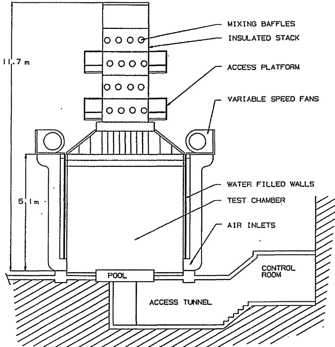
Figure 5. Arrangement of Smoke Emissions Reduction Facility (SMERF)
