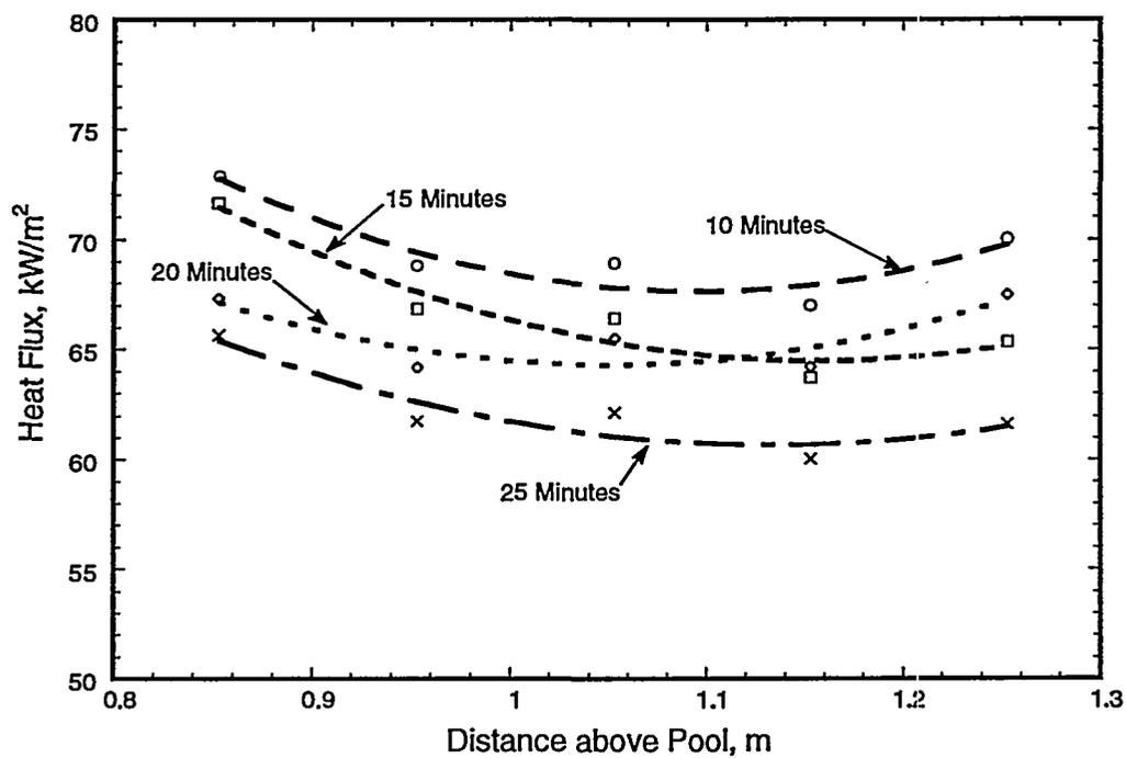
Figure 7. Heat flux data from cooled plate calorimeter in an outdoor fire.
