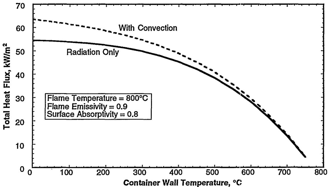
Figure 1. Heat fluxes implied by 10CFR71.
