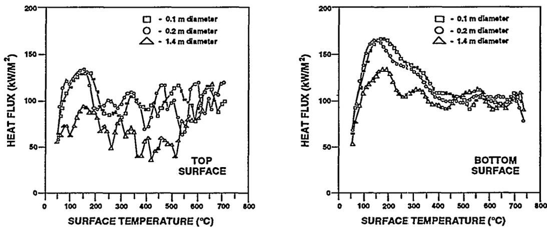
Figure 2. Cold wall heat fluxes measured in pool fire for various sized cylinders<sup>14</sup>.
