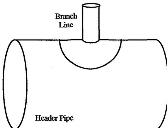
Figure 5. Certain branch lines are decoupled from the header system analytical model.
