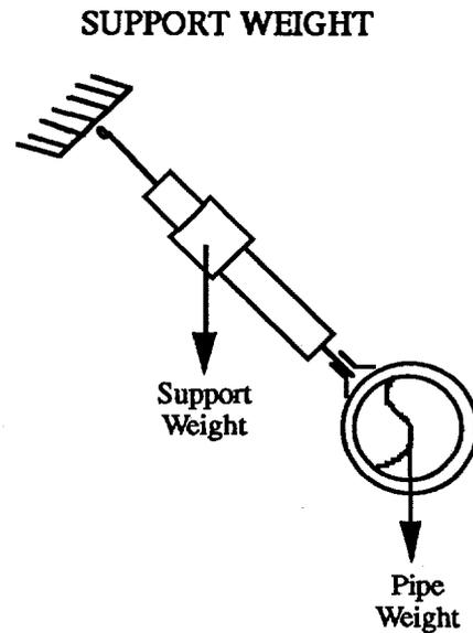
Figure 4. In certain cases part of the support weight is carried by the pipe.
