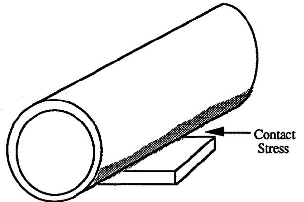
Figure 1. Local stresses at pipe - support interface
