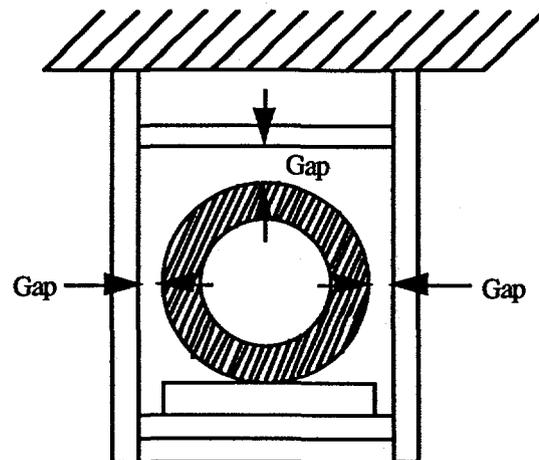
Figure 3. Small gaps can exist around the pipe in the restrained direction
