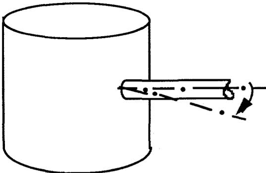
Figure 7. Equipment nozzles and shells have flexibilities which can reduce pipe reaction loads.
