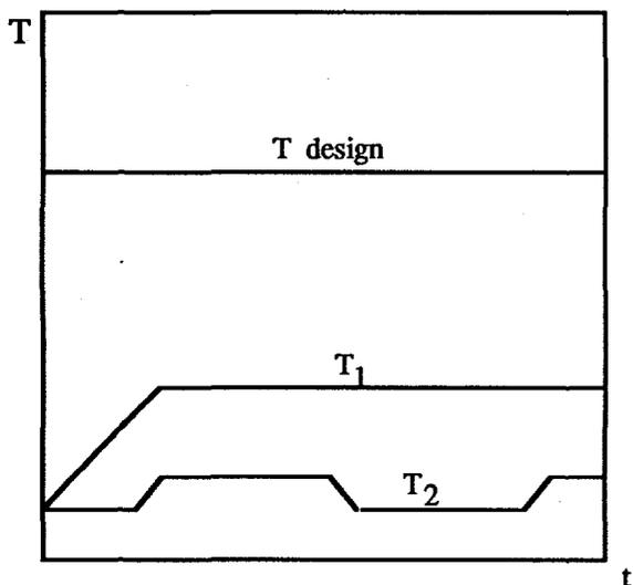
Figure 6. The Design Temperature may be set significantly higher than actual system operating temperatures.
