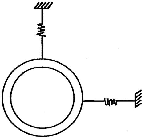
Figure 2. Supports are modeled as spring stiffnesses
