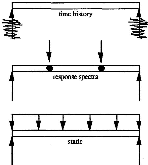
Figure 8. Applied loadings for various analytical methods.
