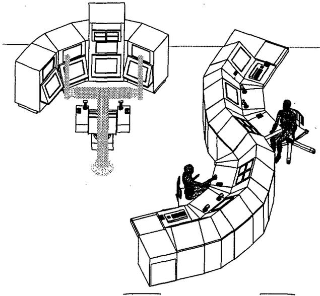
Figure 1. chief operator's, monitor's, and dexterous manipulator workstations.
