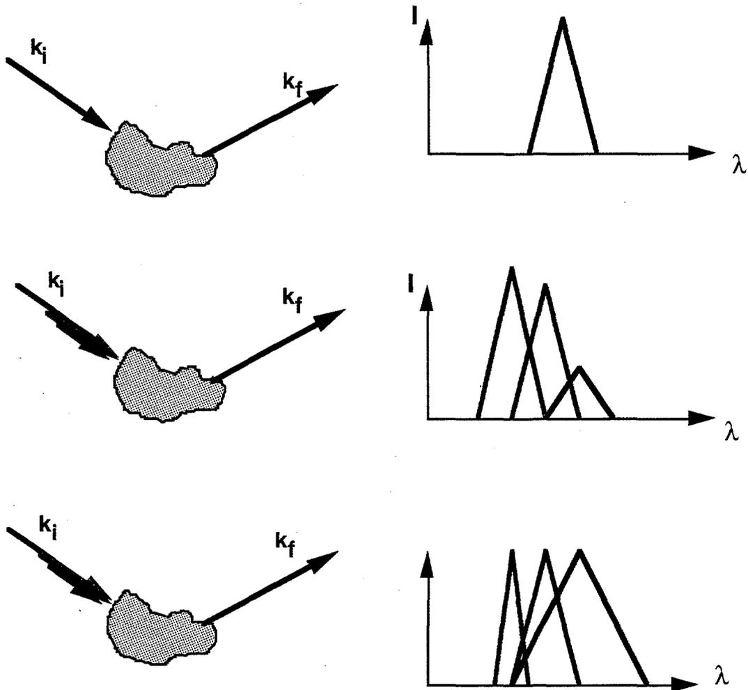
Figure 3: The upper panel represents a generic experiment using monochromatic neutrons with a particular wavelength spread. The second panel indicates that when different incident neutron wavelengths are used, the incident neutron flux may not be the same for each incident wavelength. In the lower panel an experiment is performed with different incident wavelengths but the resolution varies with that wavelength across the wavelength band used.
