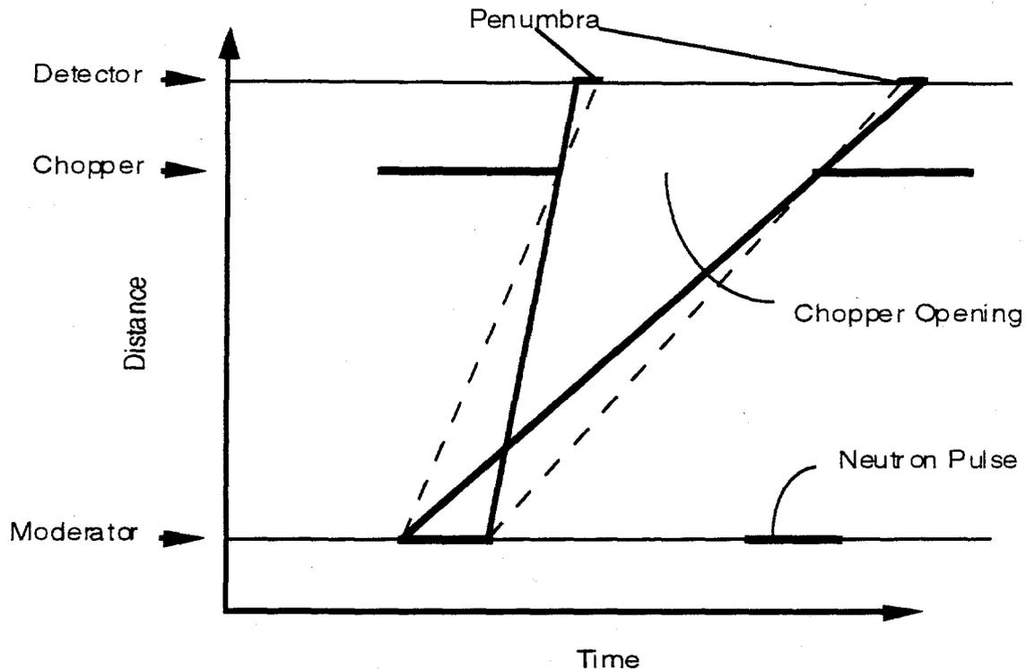
Figure 6: Distance-time diagram for a typical spectrometer. The vertical axis represents distance from the neutron source while the horizontal axis is time. The band-defining chopper results in a significant penumbra at the detector for a LPSS because the pulse duration is 5 - 10% of the time between pulses.
