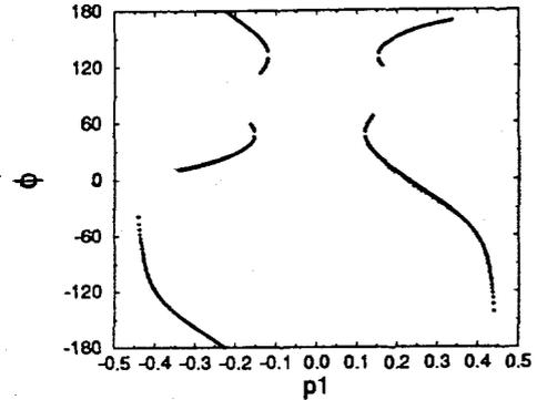
Figure 4. The relationship between the spin direction angle after the rotator, and the field  $p_1$  of the first magnet.
