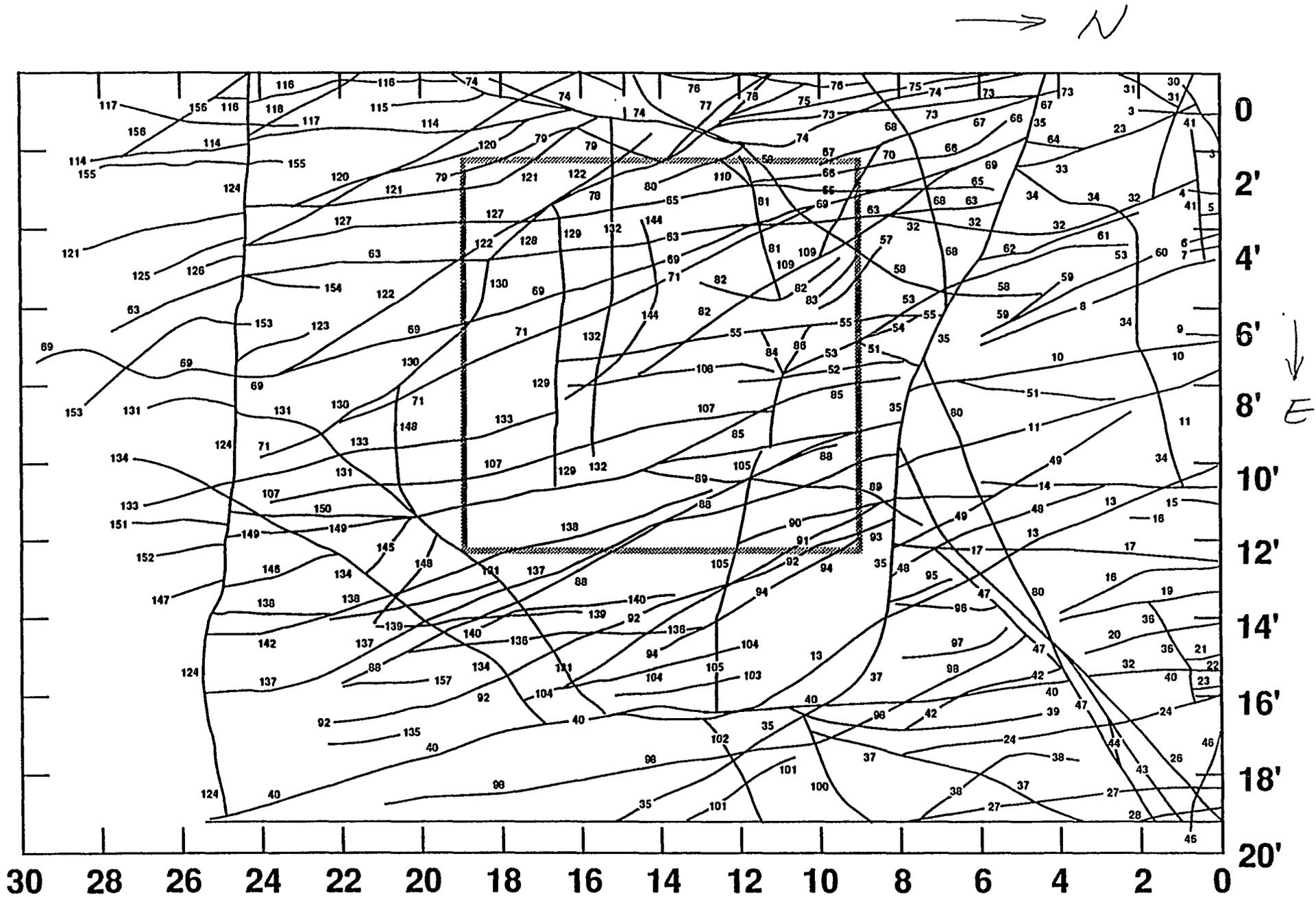
Figure 6. A map of the fractures on the ground before the sawing of the block boundary slots started. The square is the location of the large block.
