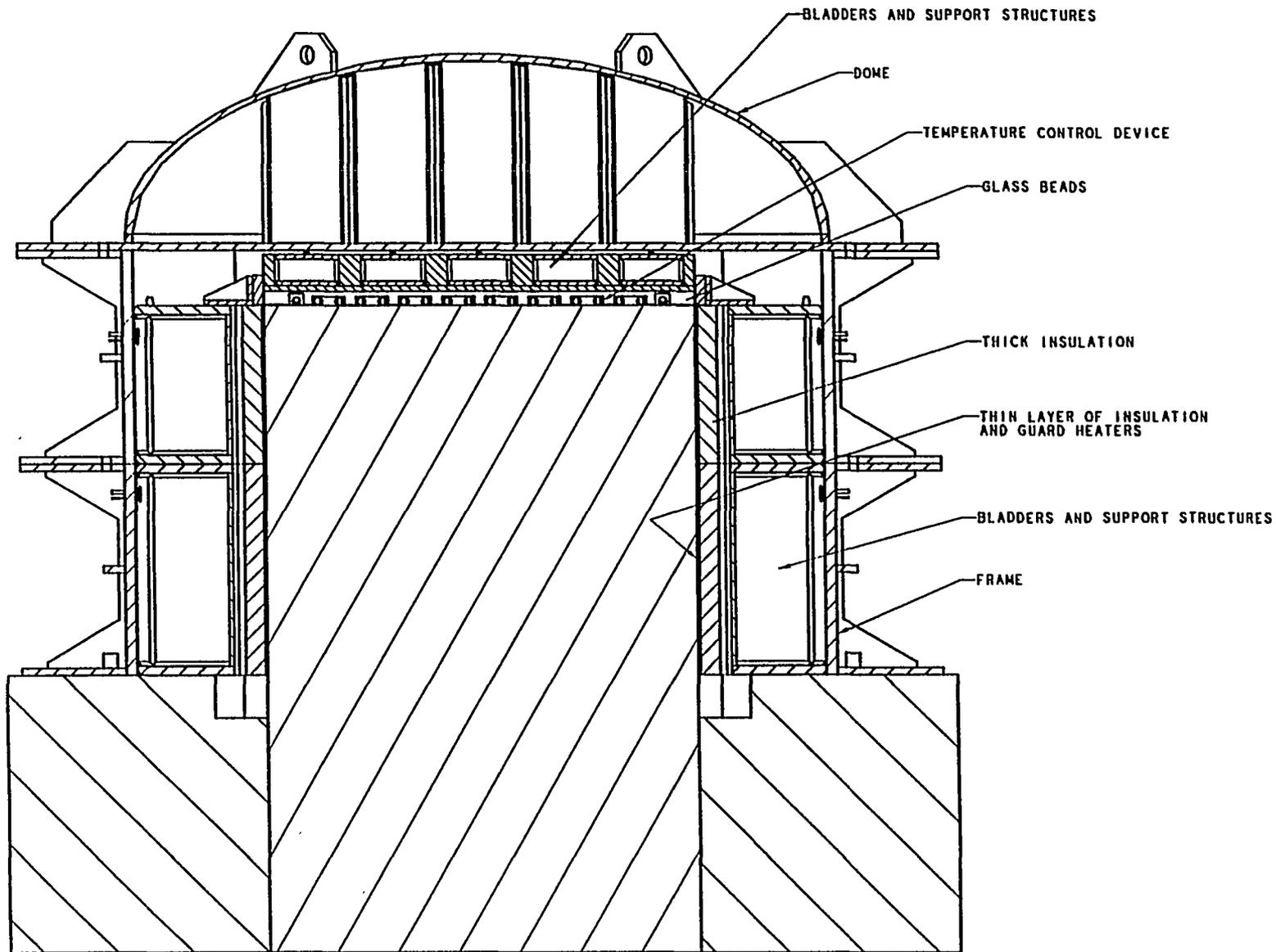
Figure 3. A schematic diagram showing the horizontal boundary control structures between the block and the frame and the vertical boundary control components on the top of the block.
