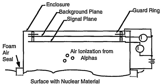
Fig. 2. An electrostatic LRAD as a (soil) surface monitor. No airflow is required in this LRAD. The ions produced by emitted alpha particles are electrostatically attracted to the signal plane. The ion current is read out by the electrometer. The guard plane reduces leakage currents through the electrometer by a factor greater than  $10^5$ .
