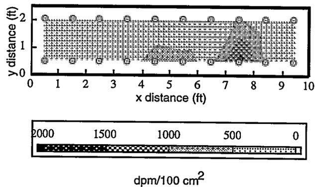
Fig. 6. Contamination levels on a stainless steel countertop at Los Alamos. Comparison data have not yet been taken..
