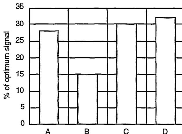
Fig. 8. Response of POM to an 1100 dpm Pu-239 source within different objects, relative to the response to the bare source. The source is placed in a hole inside an aluminum block, without (A) and with (B) a cap over the source. The source is also placed within (C) a square aluminum tube and (D) a mock NIM module.
