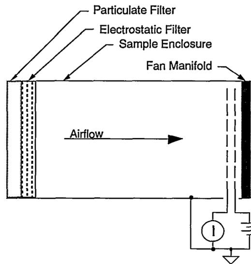
Fig. 3. Schematic of an airflow LRAD in an object monitor configuration. Filtered ambient air is drawn over the object to be monitored (not pictured) by the fans. The ions produced by emitted alpha particles are
