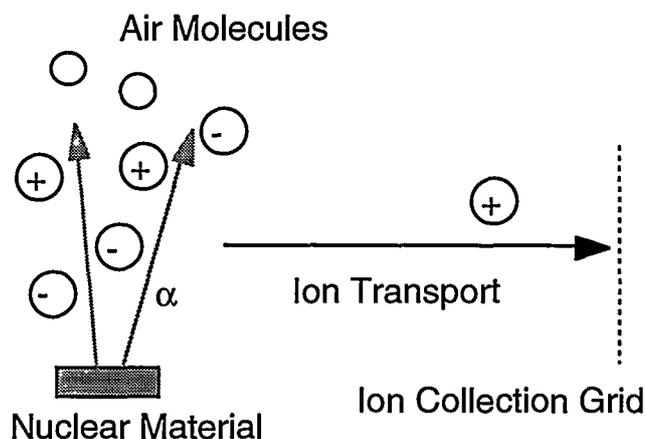
Fig. 1. Long-range alpha detection via the ions produced in air.
