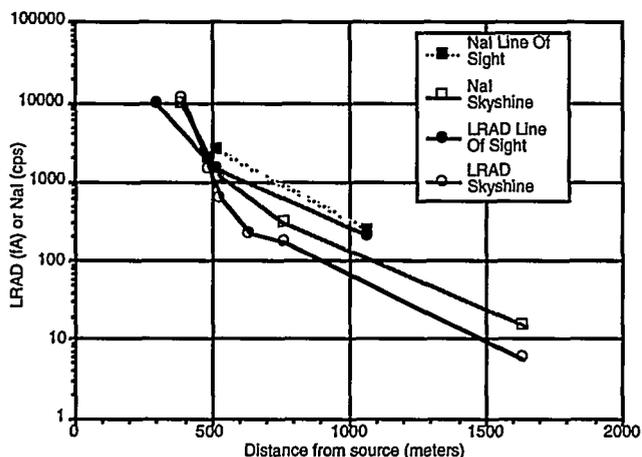
Fig. 11. Response of a mock LRAD gamma-ray monitor and a NaI detector at different distances from a gamma-ray source (a critical assembly).
