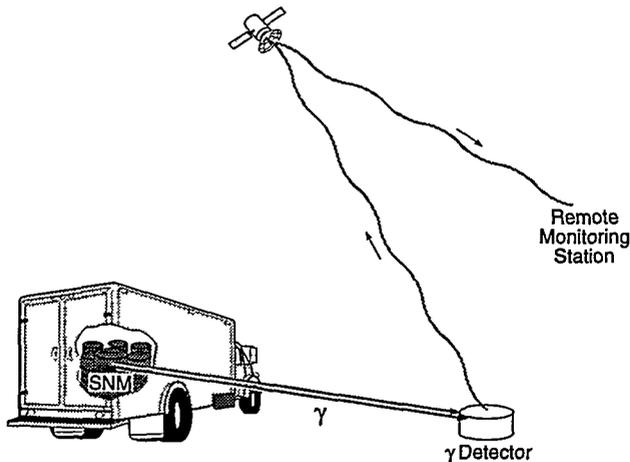
Fig. 10. Conceptual view of gamma ray monitoring at borders or other checkpoints. At the site depicted, the monitor is unattended and so alarms due to nuclear material passing nearby are relayed via satellite to remote stations.
