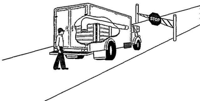
Fig. 12. Conceptual drawing of truck monitoring. The gross ionization detector is placed briefly within the open volume of a cargo space. Air is circulated through the chamber. Ideally, if alpha-emitting nuclear material is located on any surfaces within the volume, the equilibrium ion concentration will be greater than typically found.
