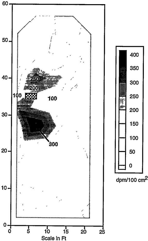
Fig. 4. Comparison of small surface LRAD monitor with spot results from a conventional hand-held survey meter. Results obtained on an old blasting pad at Los Alamos National Laboratory.
