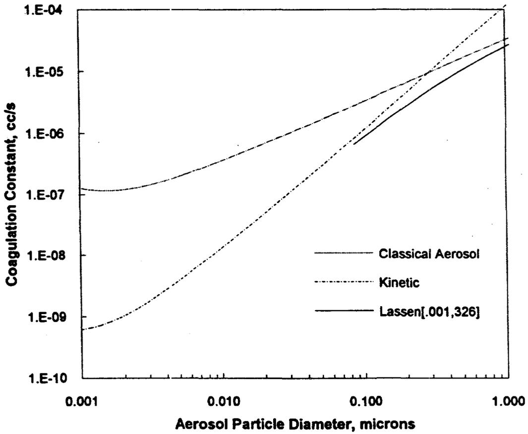
Figure 3. The Lassen and Rau attachment model bridges other coagulation theories in the submicron aerosol region.
