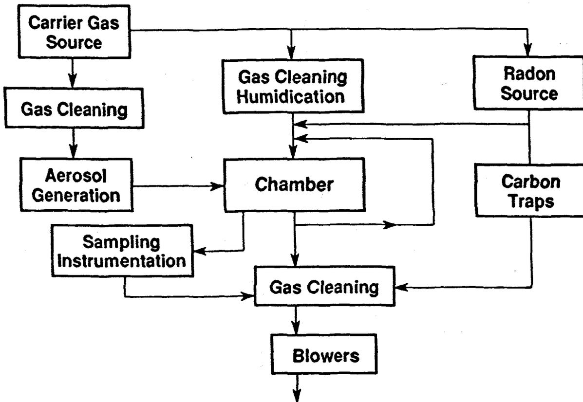
Figure 4a. Radon progeny attachment studies are performed using this experimental configuration.
