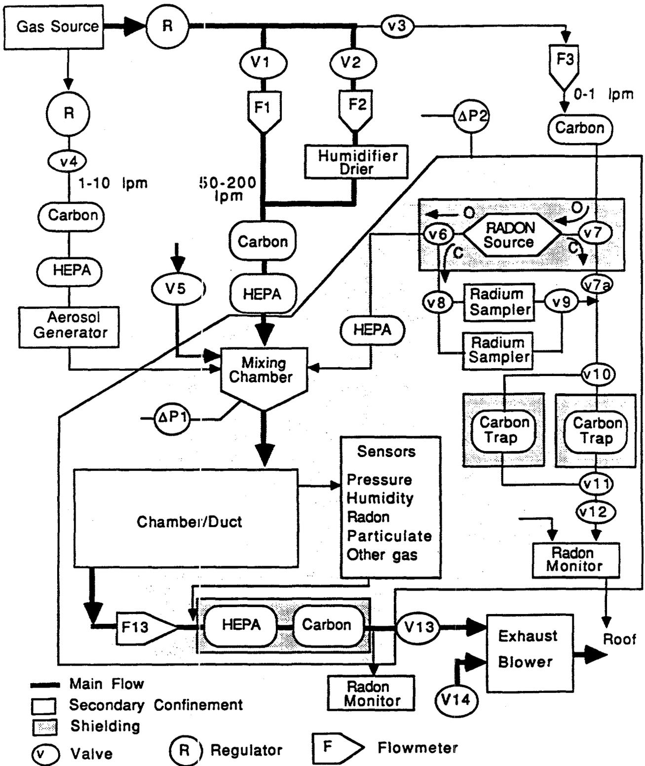
Figure 4b. Diagram of the Experimental Flow System.
