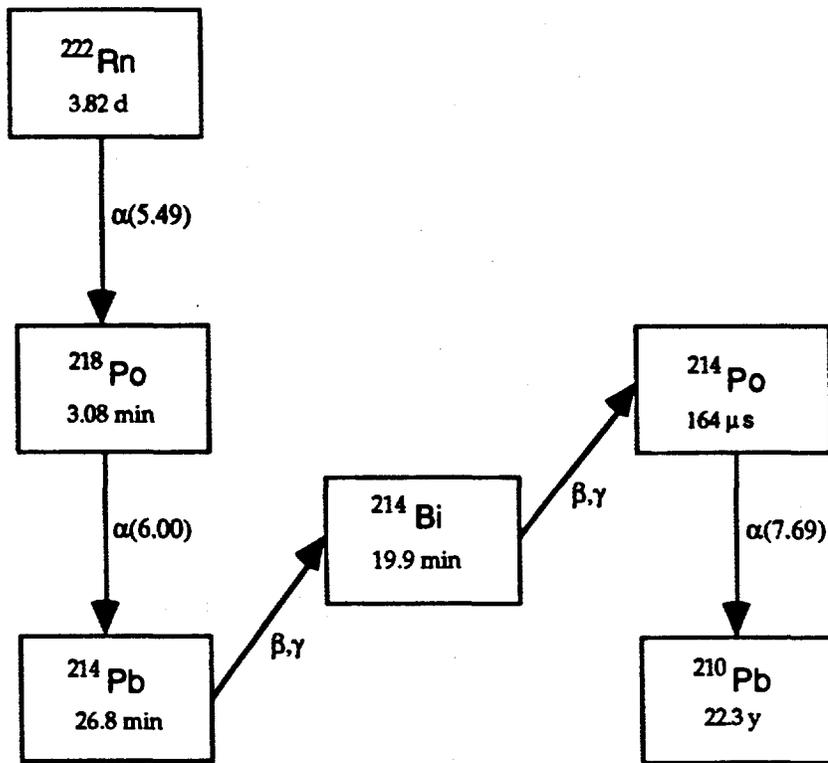
Figure 2. The radioactive decay scheme for radon and its daughters (through  $^{210}\text{Pb}$ ). Half lives and alpha decay energies (MeV) are indicated.
