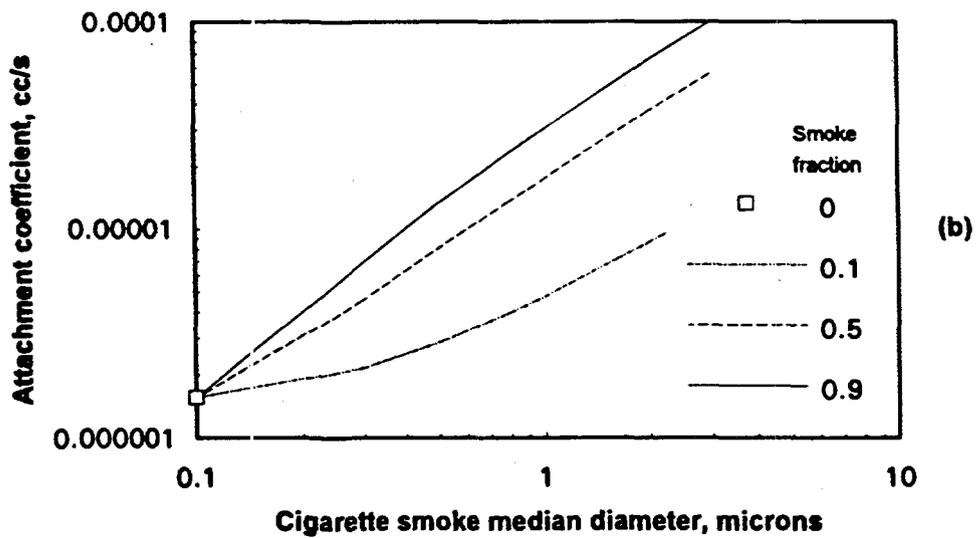
Figure 14. (a) The overall attachment rate of radon progeny to an aerosol increases with the median size and the standard deviation characterizing the aerosol distribution. (b) In the presence of a fixed ambient aerosol, increases in the attachment coefficients also result with increased proportions of the cigarette smoke aerosol. The log normal parameters for the ambient aerosol were taken as  $n_m = 0.1 \mu\text{m}$  and  $\sigma_g = 2.0$ .
