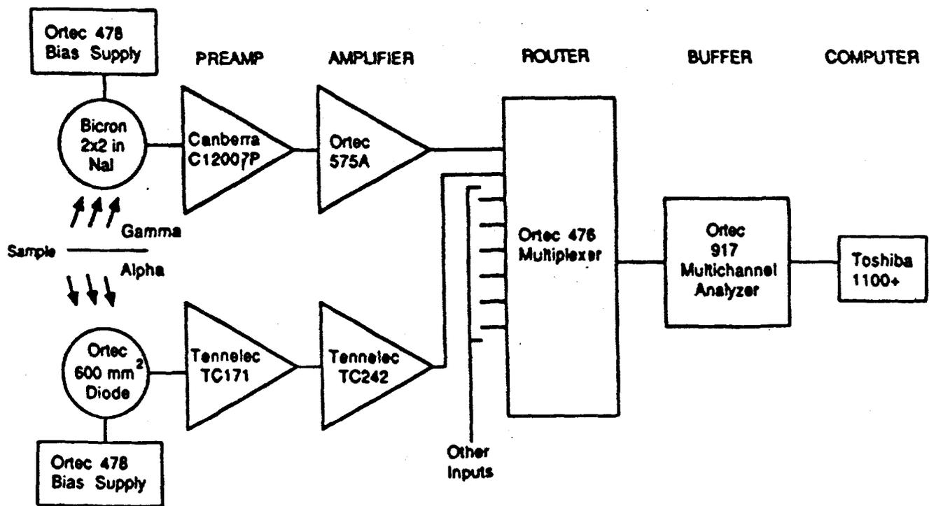
Figure 5. A block diagram of the alpha-gamma detector system.
