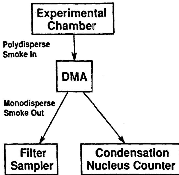
Figure 6. The differential mobility analyzer can be used for both aerosol generation and fractionation.
