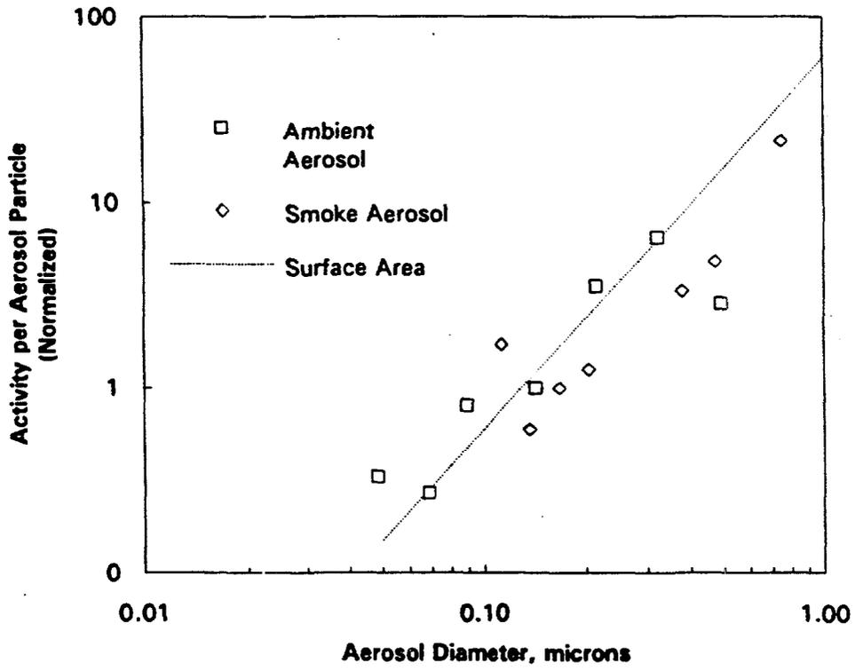
Figure 12. The behavior of radon attachment to differing particle sizes is illustrated for the cigarette smoke and the laboratory room aerosols.
