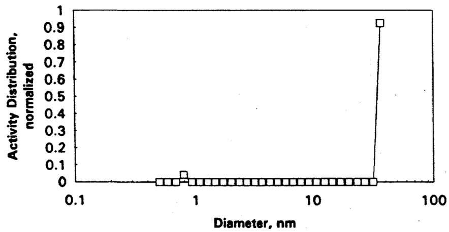
Figure 9. In the presence of a smoke aerosol, the graded-screen diffusion battery indicates a bimodal Po-218 activity distribution.
