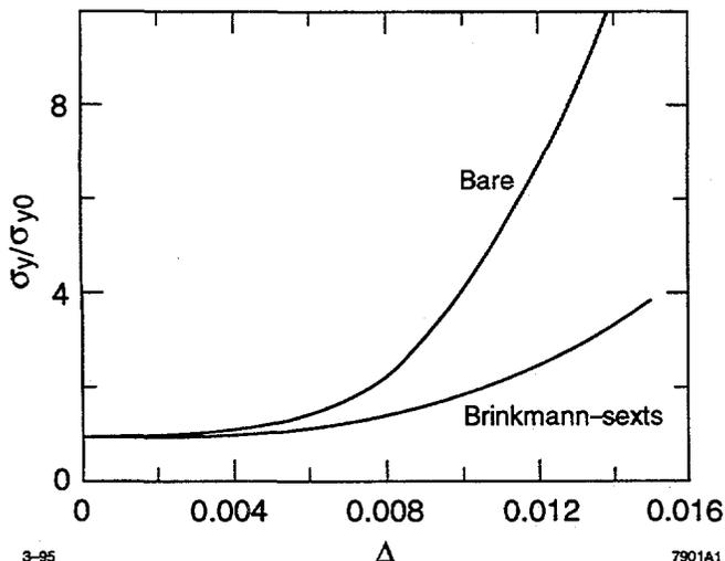
Figure. 1. Comparison of relative increase of vertical spot size with and without Brinkmann-sextupoles as a function of the half-width  $\Delta$  of a uniform momentum distribution, for  $\beta_x^* = 37$  mm and  $\beta_y^* = 100$   $\mu$ m. Synchrotron radiation effects not included.
