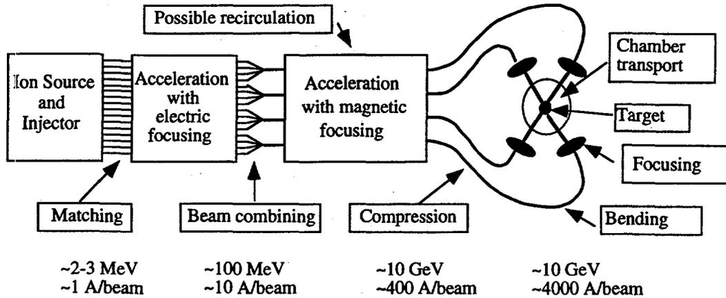
Fig. 4. Schematic of a “conventional” induction accelerator driver.
