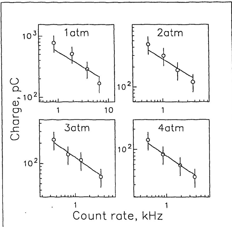
Fig. 6: Average charge in an event versus the tube count rate at different gas pressures
