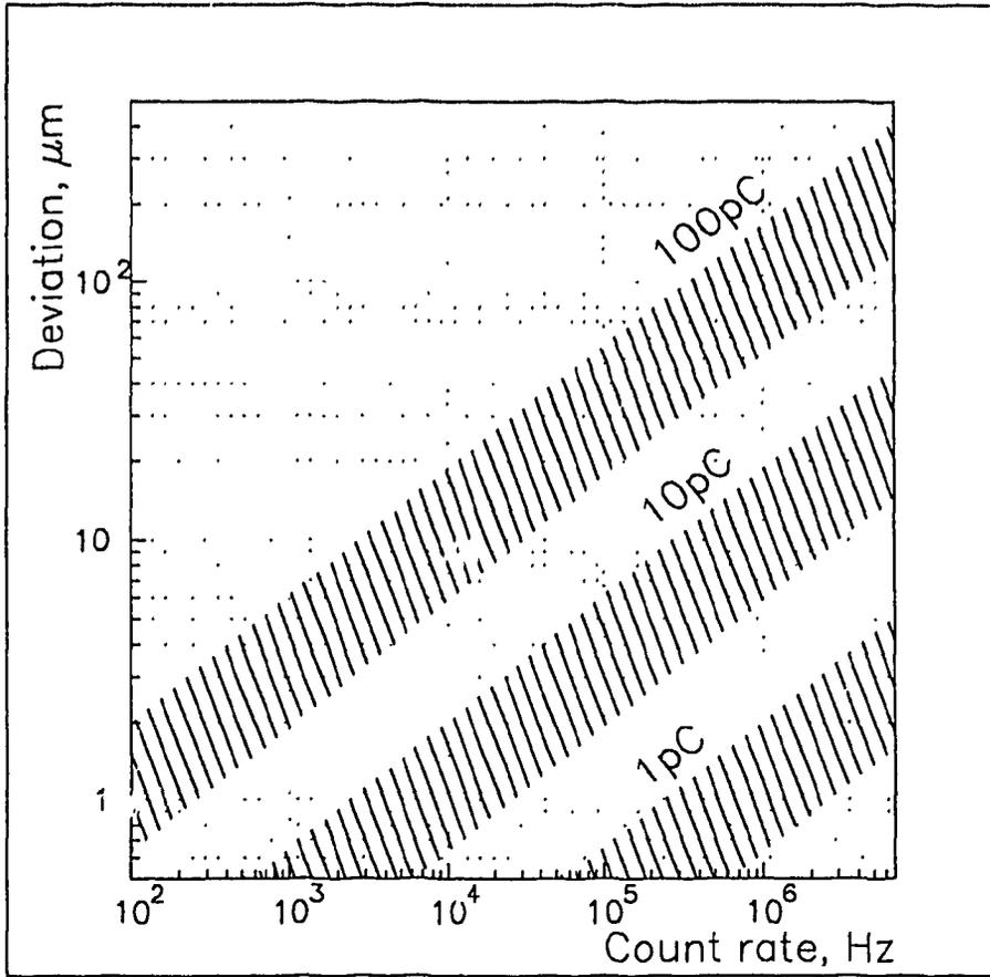
Fig. 2: The calculated average vibration amplitude versus the count rate
