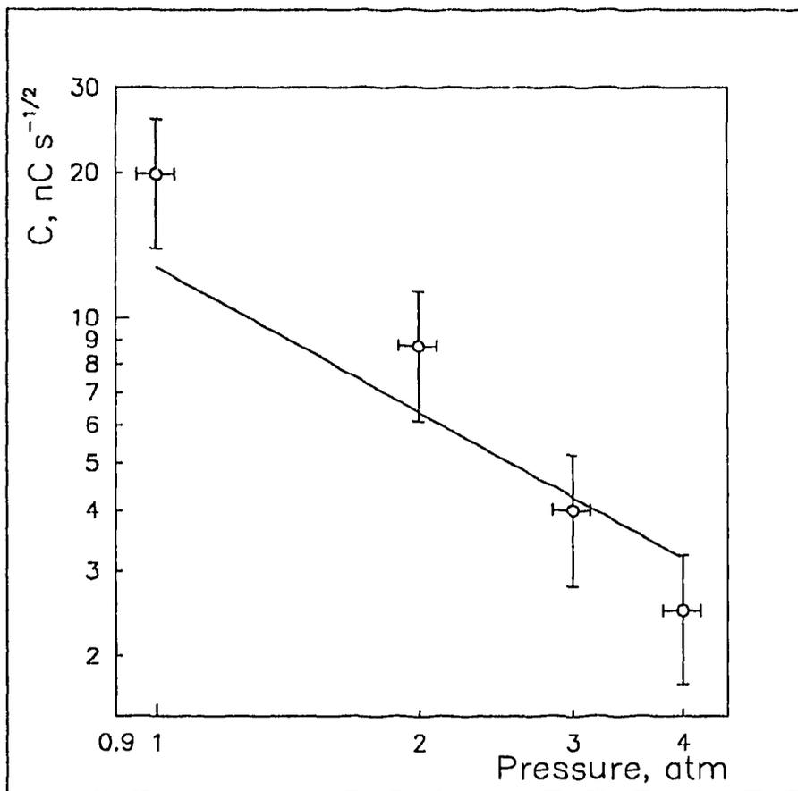
Fig. 7: The product of the charge and the square root of the count rate measured at fixed vibration amplitude as a function of the gas pressure
