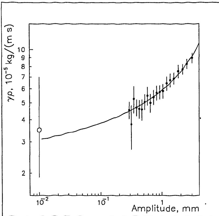
Fig. 8: The  $\gamma\rho$  value versus vibration amplitude in the air. Empty circle shows the value obtained from the data of the wire vibration in the tube
