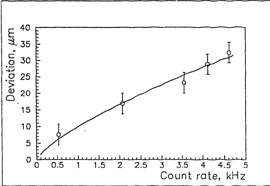
Fig. 5: Vibration amplitude as a function of the detector count rate
