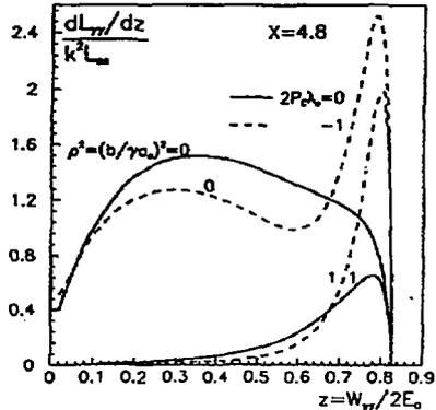
Figure 2: The spectral luminosity of  $\gamma$ - $\gamma$  collisions. The curves represent unpolarized electrons or photons and fully polarized photons on helicity unity electrons. Two different distances between the conversion point and the collision point are considered. [From V. Telnov, Nucl. Instrum. Methods A355, 3 (1995)].
