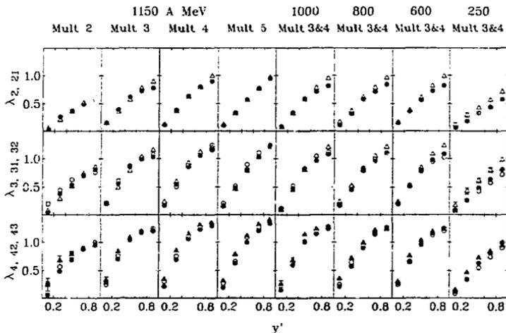
Figure 4: Sideward flow parameters  $\lambda$  as a function of rapidity. The open triangles indicate  $\lambda_{A1}$ , the parameter based on the  $A$ th power of the proton spectrum. The solid circles indicate both  $\lambda_2$ , the parameter for deuterons, and  $\lambda_{A2}$ , the parameter for the deuteron spectrum to the power of  $A/2$ . Likewise, the open circles indicate  $\lambda_3$  and  $\lambda_{A3}$ , and the solid triangles indicate  $\lambda_4$ .
