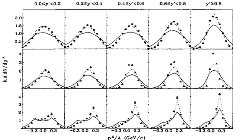
Figure 3: Data for Mult 4 collisions of 1.15A GeV Au + Au, showing relative  $p^x/A$  density for deuterons (circles) and  $\alpha$  particles (triangles); the dashed curves are proton density squared and the dotted curve are deuteron density squared. The usual condition  $p^x/A \geq 0.2$  GeV/c has been applied to the lower row of panels only.
