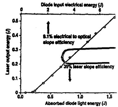
Fig. 14. Efficiency of Yb:S-FAP DPSSL.
