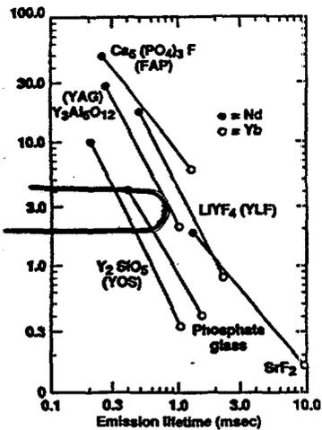
Fig. 2. Comparison of storage times and gain cross section for materials doped with Nd and with Yb.
