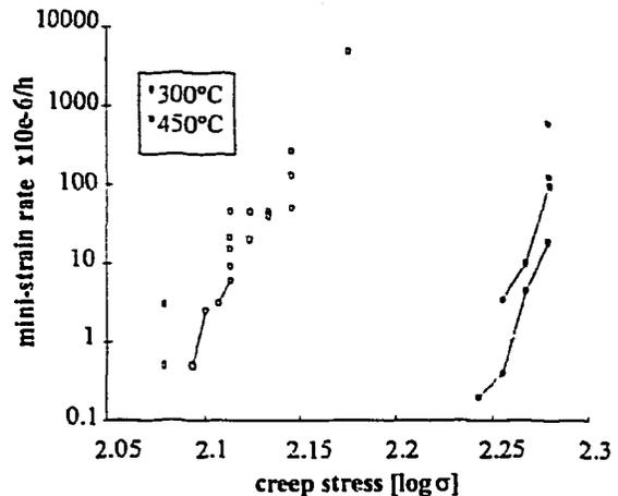
Figure 5 : Stress dependance of creep strain. Creep tests at 450°C and 300°C.
