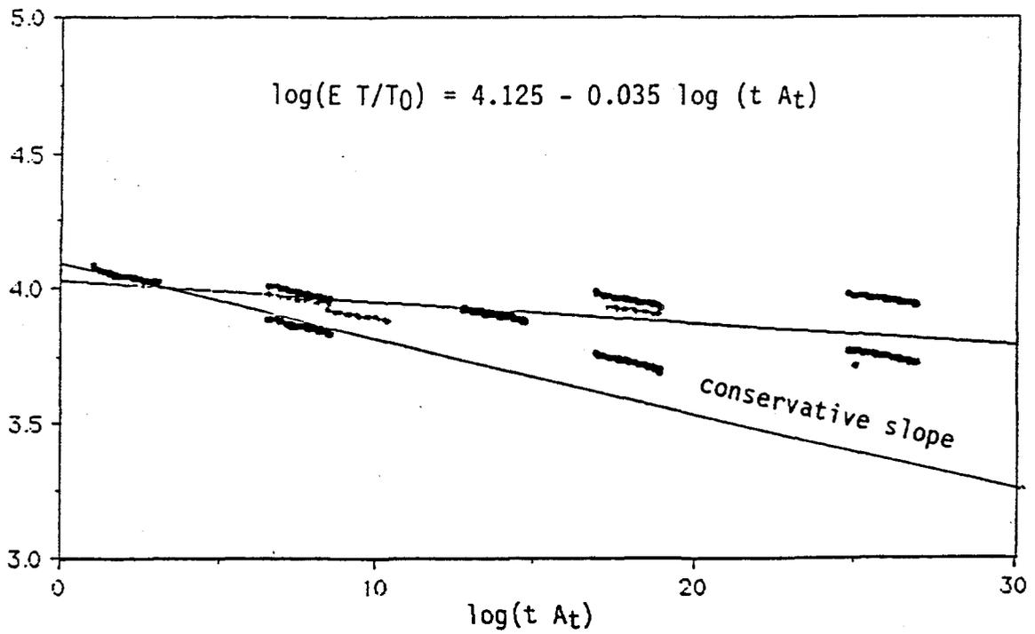
Figure 3.2. Master Curve for Creep of HDPE: Conservative Slope
