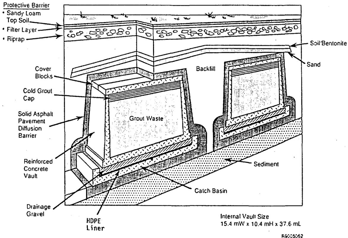
Figure 1.1. Schematic of Grout Vault Design With Liner in Catch Basin
