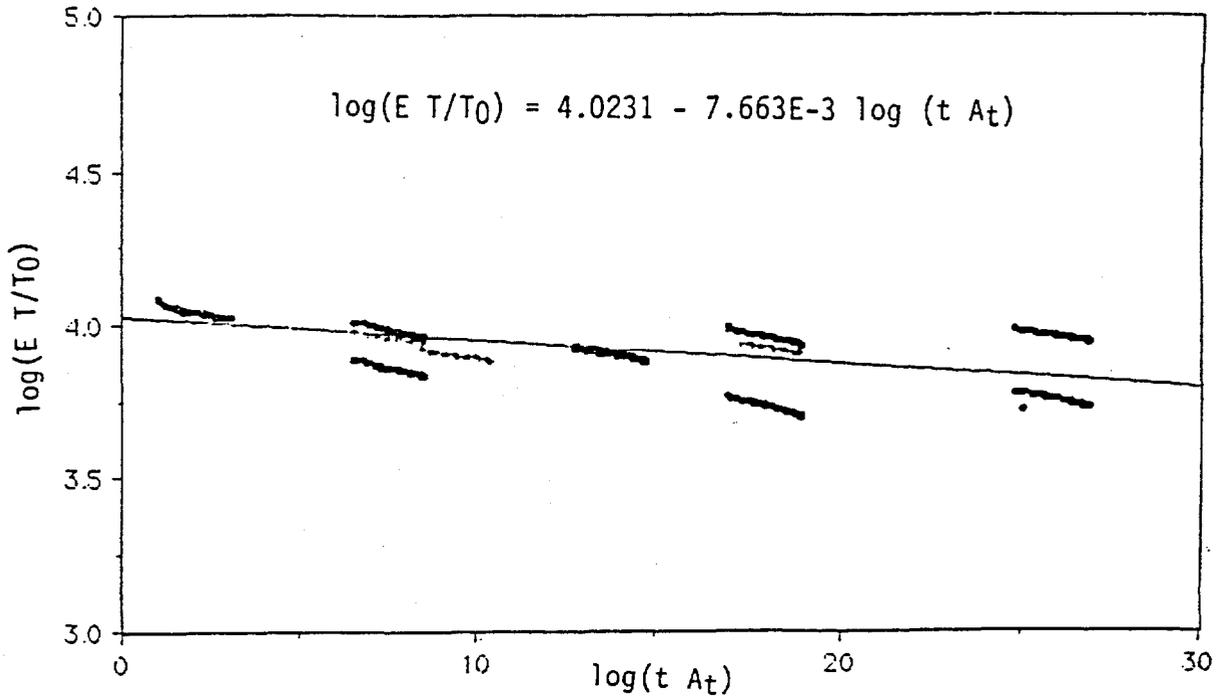
Figure 3.1. Master Curve for Creep of HDPE: Best Fit Slope
