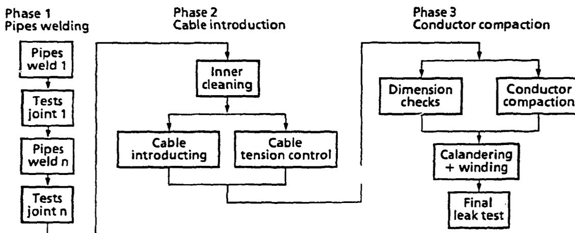
Figure 2. Block diagram of the jacketing line
