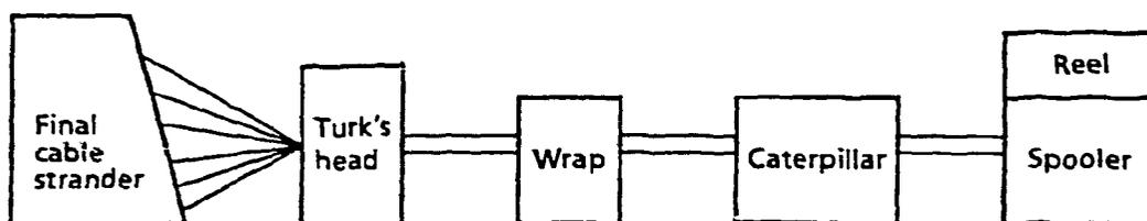
Figure 1. Block diagram of the cabling line
