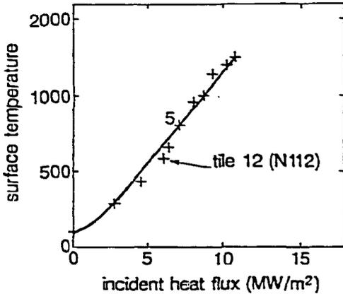
Figure 5. Surface temperature of N112 versus the incident heat flux
