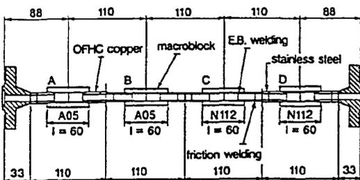
Figure 7. Divertor mock-up made of 4 blocs
