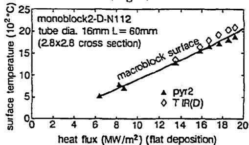
Figure 9. Surface temperature versus heat flux
