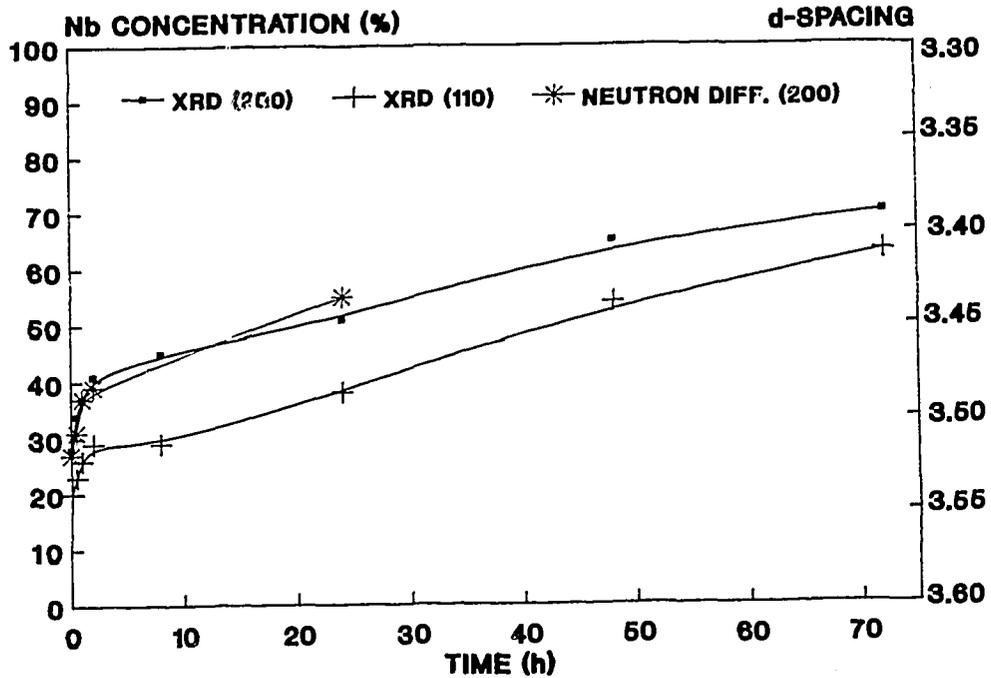
Figure 8 Comparison of d-spacing for RN(200) and LN(110) diffraction from the  $\beta$ -phase in Zr-2.5 wt% Nb pressure tube material as a function of time during heat-treatment at 400°C (autoclaving temperature) [5].
