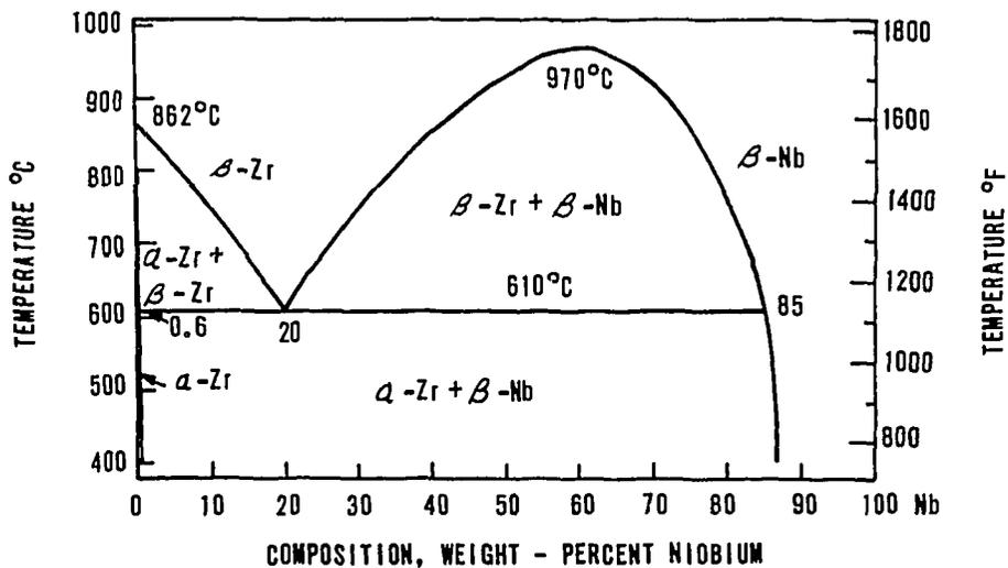
Figure 3 The zirconium-niobium phase diagram [1].
