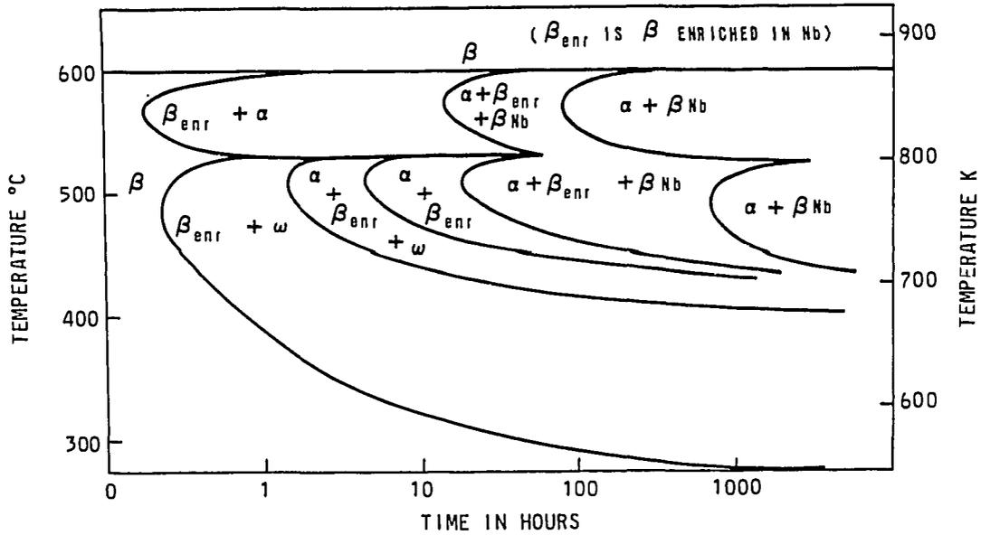
Figure 7a TTT-diagram for a Zr-19 wt% Nb alloy [2].
