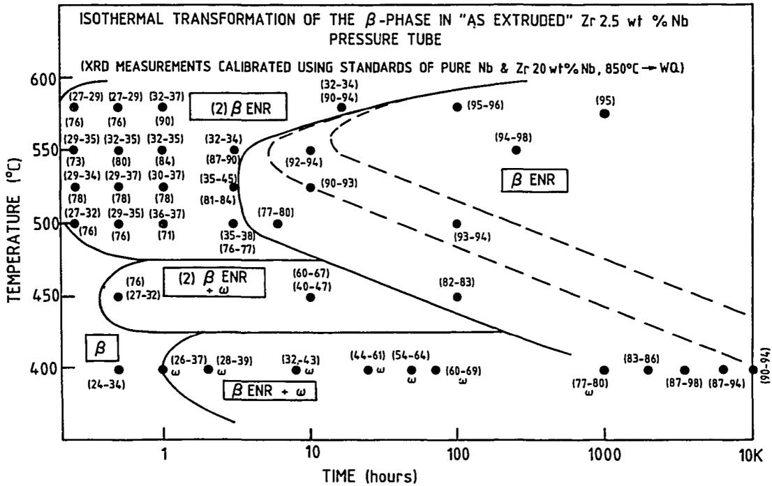
Figure 7b TTT-diagram for a Zr-2.5 wt% Nb pressure tube. The numbers in brackets refer to Nb concentration. For two discrete  $\beta$ -phase components there are two bracketed values. Where two numbers are shown in one bracket the values refer to measurements using the (110) and (200) planes, see text.
