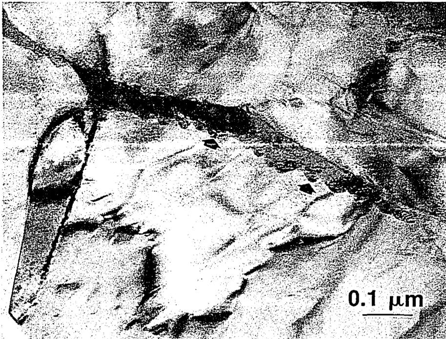
Figure 9 Electron micrograph showing  $\beta$ -phase filament in pressure tube H737 after heat-treatment for 1 h at 500°C. There is no evidence for  $\omega$ -phase, although some Nb-rich precipitates are observed at the  $\alpha/\beta$  interface (arrowed).
