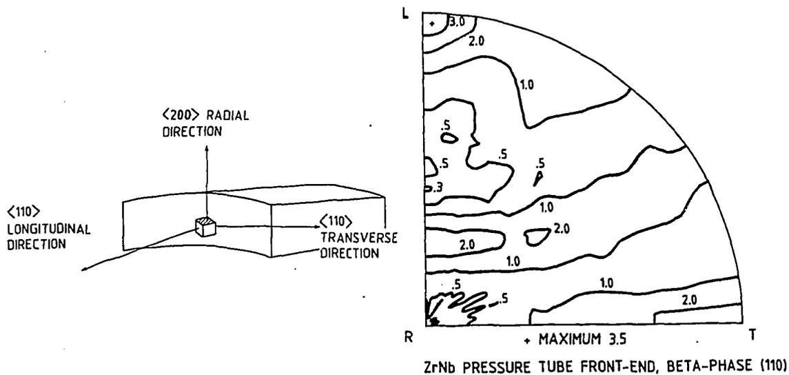
Figure 4 Quarter (110) pole figure and schematic diagram illustrating preferred orientation of the  $\beta$ -phase in Zr-2.5 wt% Nb pressure tubes.
