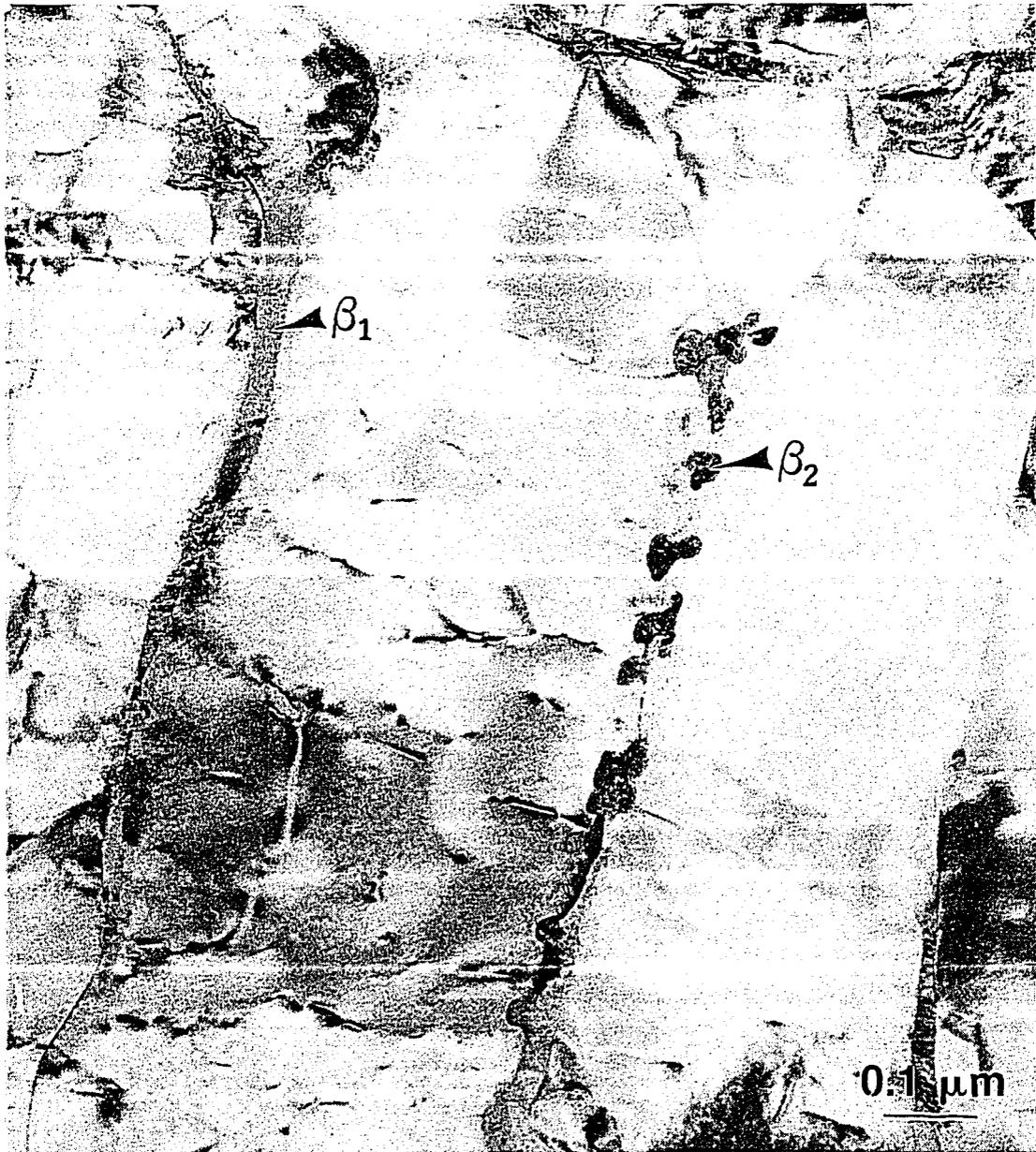
Figure 13 Electron micrograph showing the state of the  $\beta$ -phase in pressure tube H737 after heat-treatment for 1 h at 550°C. Nb-rich precipitates are formed at the  $\alpha/\beta$  interface or from completely decomposed (discontinuous)  $\beta$ -phase ( $\beta_2$ ). Other segments of  $\beta$ -phase remain relatively intact ( $\beta_1$ ).
