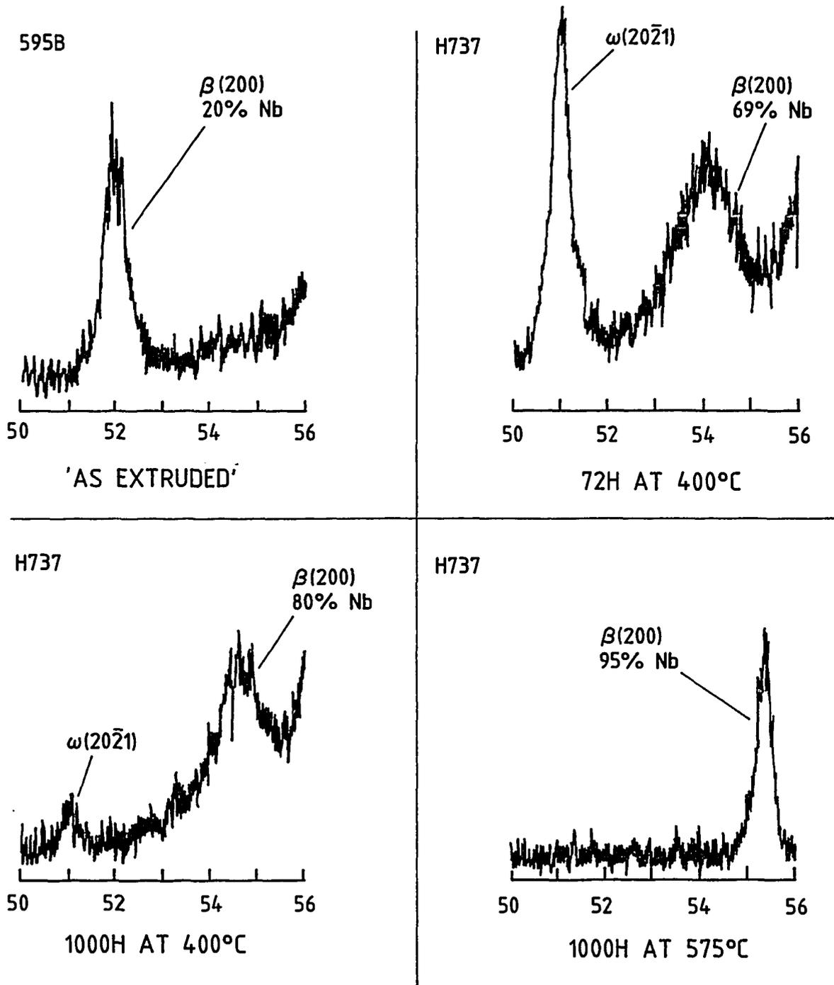
Figure 6 Diffractometer scans of radial-normal specimens after various thermal treatments showing the  $\beta(200)$  and  $\omega(20\bar{2}1)$  line profiles.
