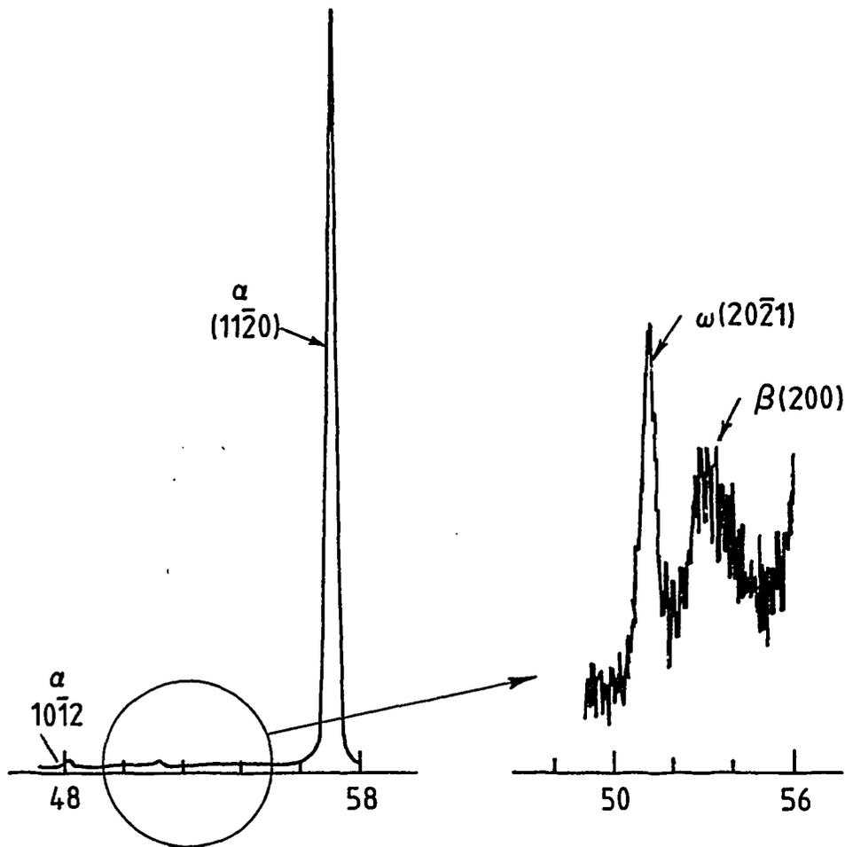
Figure 2 Diffractometer scans from a radial-normal specimen of cold-worked Zr-2.5 wt% Nb pressure tube H737 given 24 h at 400°C, showing the relative intensities of  $\alpha$ ,  $\beta$ , and  $\omega$ -phase reflections. The diffraction angles are shown on the bottom scale. Peaks for  $\omega$  (20 $\bar{2}$ 1) and  $\beta$ (200) correspond with diffraction angles ( $2\theta_B$ ) of about 51° and 53°, respectively [2].
