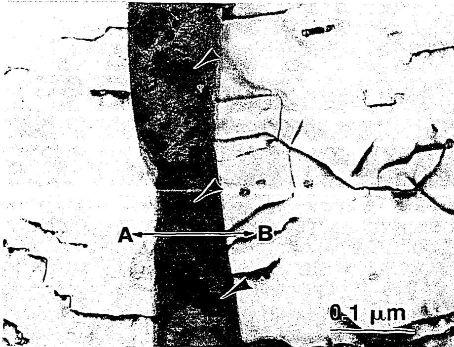
Figure 12 Micrograph and composition profile for  $\beta$ -phase in a Zr-2.5 wt% Nb pressure tube after heating for 24 h at 400°C. The filament contains  $\omega$ -phase particles (arrowed), and there is segregation of Nb and Fe at the  $\alpha/\beta$  interface.
