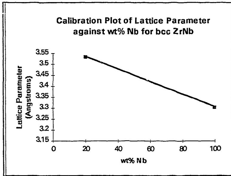
Figure 5 Calibration plot of bcc lattice parameter versus wt% Nb for ZrNb at 25°C.
