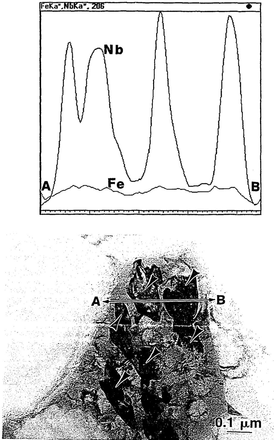
Figure 10 Micrograph and composition profile for  $\beta$ -phase in Zr-2.5 wt% Nb after heating for 1 h at 700°C and then for 1 h at 500°C. There is a denuded zone of  $\omega$ -phase particles (arrowed) at the  $\alpha/\beta$  interface. The  $\omega$ -phase is depleted, and the  $\beta$ -phase is enriched, in Nb and Fe.
