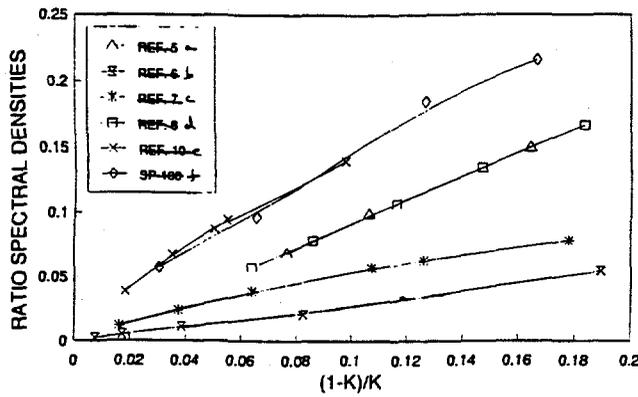
Fig. 1. Ratio of spectral densities versus  $(1 - k)/k$  for a variety of fissile systems.
