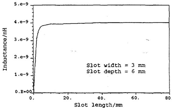
Figure 4. Inductance as a function of slot length.
