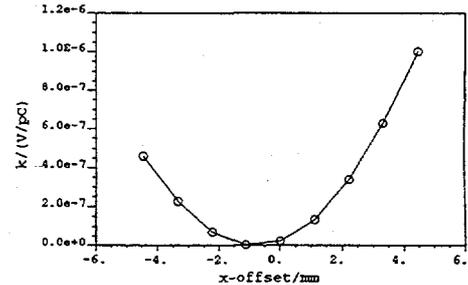
Figure 10. The longitudinal loss parameter as a function of horizontal position  $x$ . The functional dependence is nearly quadratic. Due to the mechanical asymmetry, the minimum of the wake is not at the center  $x=0$ , but is slightly shifted away from the slotted side of the vacuum chamber.
