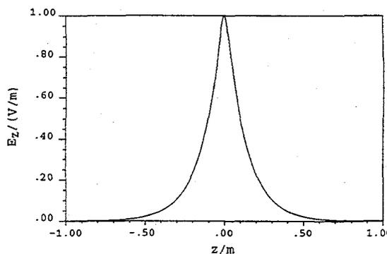
Figure 2. Longitudinal component of the electric field of the trapped mode  $TM_{010}$  in a small "cavity" ( $r_{outer}=45$  mm) in a circular beam pipe. Note the exponential decay over a long distance at both sides.
