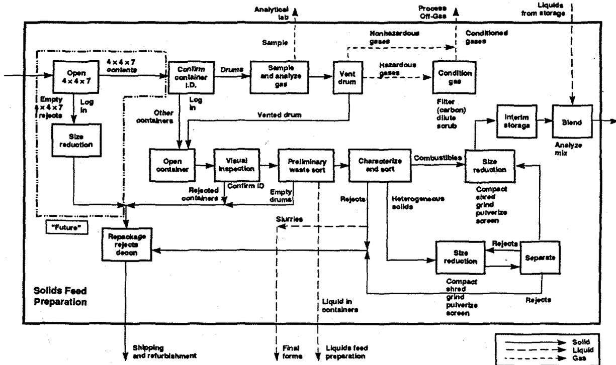
Figure 1. Functional Flow Diagram for Solids Feed Preparation
