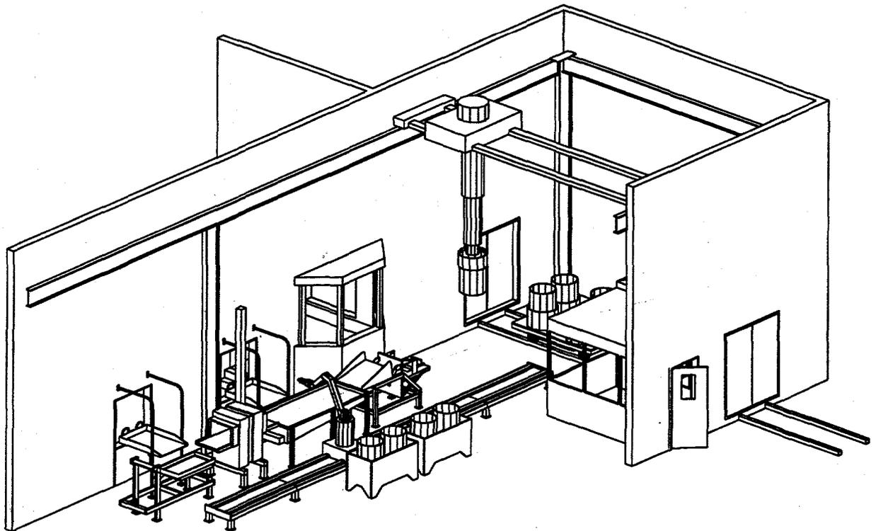
**Figure 3. 3D Representation of Receiving, Extraction and Sorting Area**
