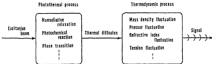
Fig. 2. Phenomenological representation of the photothermal signal generation process.
