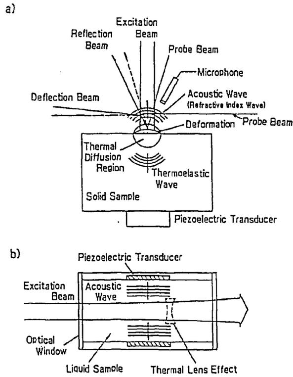
Fig. 1. Photothermal effects on and in condensed phase samples. (a) Solid sample, and (b) liquid sample [1].
