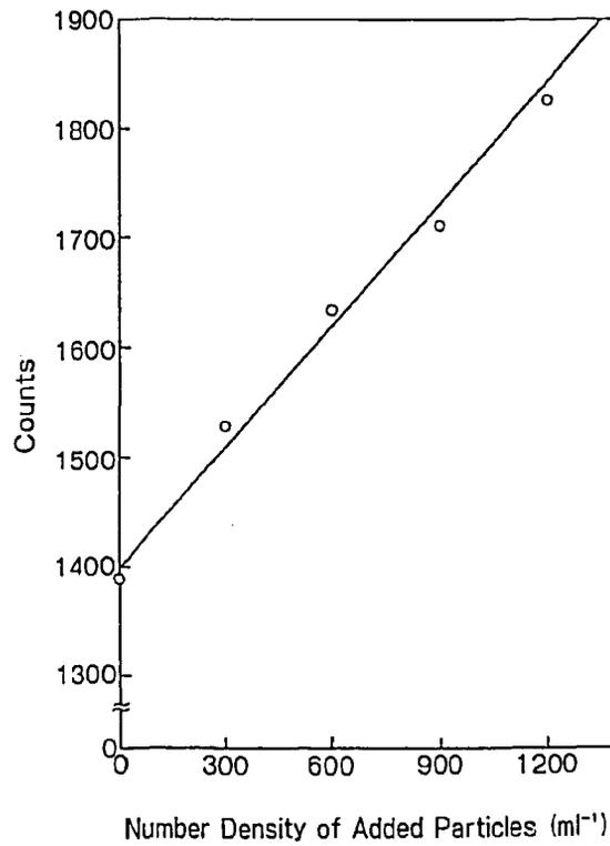
Fig. 4. Dependence of the breakdown acoustic pulse counts on the number density of the added  $0.038 \mu\text{m}$  polystyrene ultrafine particles.
