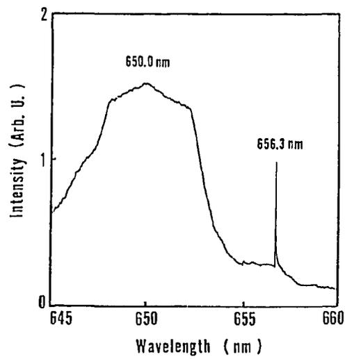
Fig. 5. Forward direction plasma emission spectrum of an underwater plasma generated from a  $0.3 \mu\text{m}$  polystyrene microsphere.
