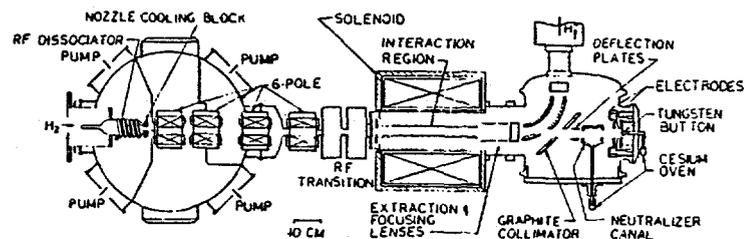
Fig. 2. Polarized H<sup>-</sup> ion source.
