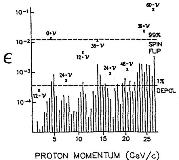
Fig. 3. Calculated resonance strength at the AGS.
