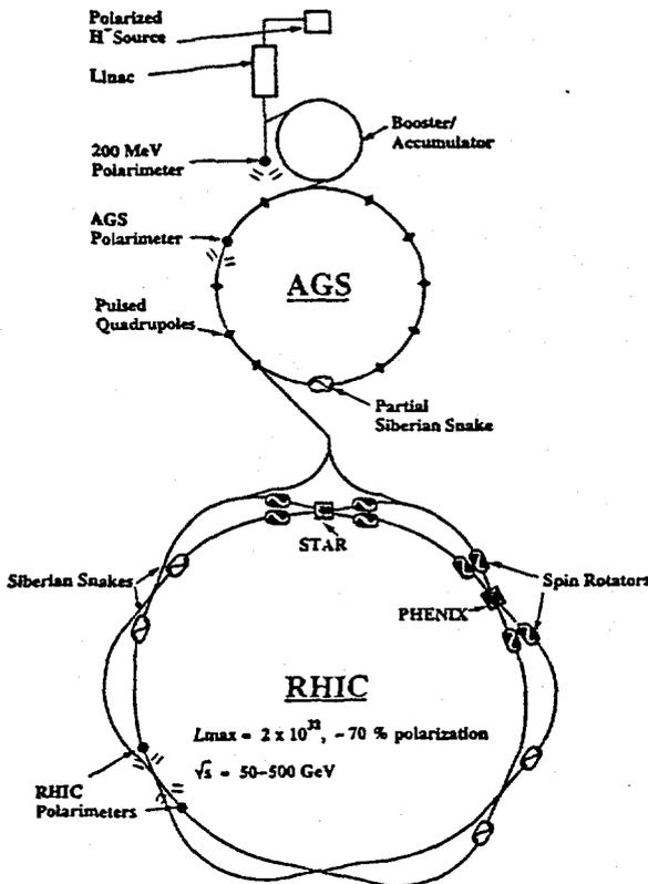
Fig. 1. Polarized proton program at BNL.
